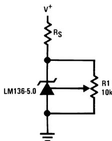
Figure 14. LM136-5.0 with Pot for Adjustment of Breakdown Voltage (Trim Range = ±1.0V Typical)
