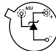
Figure 2. TO Metal Can Package (Bottom View)
