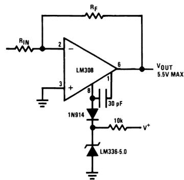
Figure 20. Op Amp with Output Clamped
