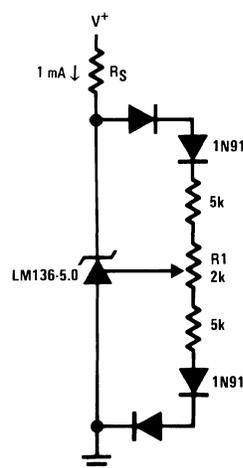
Figure 15. Temperature Coefficient Adjustment (Trim Range = ±0.5V Typical)
