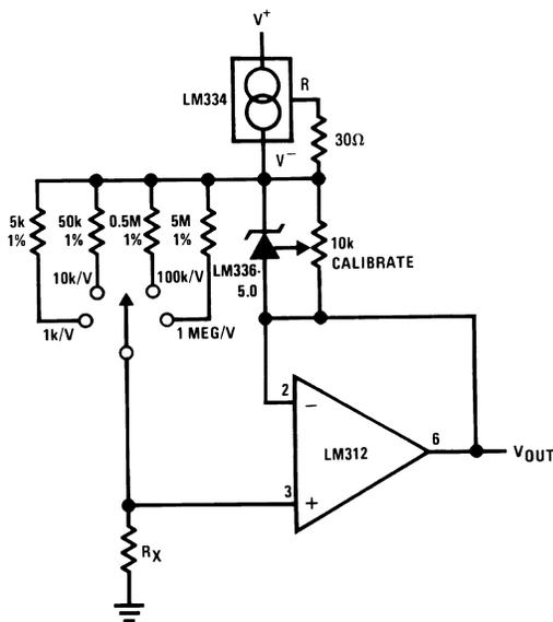
Figure 19. Linear Ohmmeter
