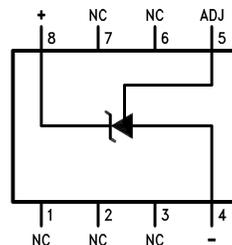
Figure 3. SOIC Package
