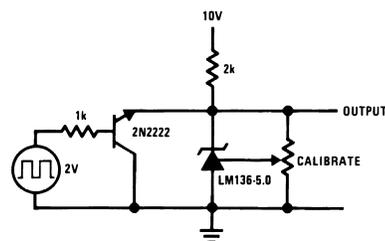
Figure 22. 5.0V Square Wave Calibrator
