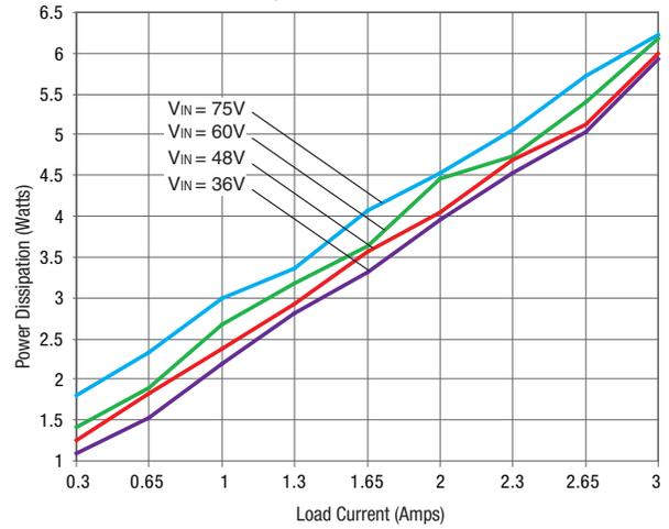
**ULE-48/1.25-D48 Power Dissipation vs. Load Current @ +25°C**
