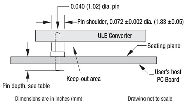
The "integral" pin shoulder is formed as part of the extruded pin fabrication and replaces the plastic standoff spacer. The shoulder diameter is 0.072 +/-0.002" and forms the mounting plane of the converter. The user should provide sufficient clearance for a 0.040" pin hole but well below the 0.072" shoulder diameter. This mounting plane avoids mechanical stress placed on the converter components. Do not place the components below the converter.
