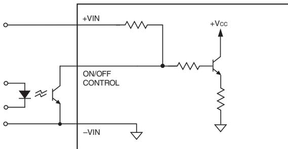
Dynamic control of the remote on/off function is facilitated with a mechanical relay or an open-collector/open-drain drive circuit (optically isolated if appropriate). The drive circuit should be able to sink appropriate current (see Performance Specs) when activated and withstand appropriate voltage when deactivated. Applying an external voltage to the On/Off Control when no input power is applied to the converter can cause permanent damage to the converter.
