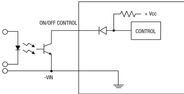
Optional Negative-polarity devices (“N” suffix) are off when the On/Off Control is open (or pulled high), and on when the On/Off Control is pulled low with respect to  $-V_{IN}$  as shown in Figure 5.
