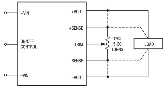
A single resistor connected from the Trim to the +Output, or +Sense where ap-
