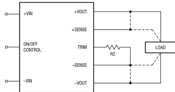
from the Trim to the –Output, or –Sense where applicable, will decrease the output voltage in this configuration.
