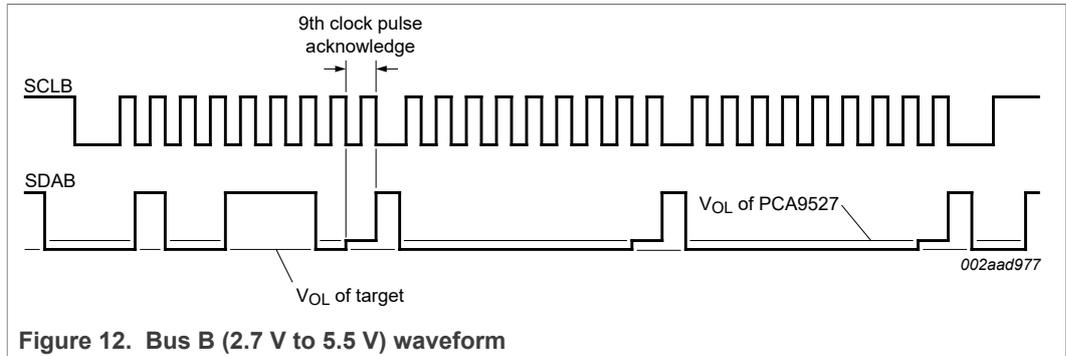
Figure 12. Bus B (2.7 V to 5.5 V) waveform
