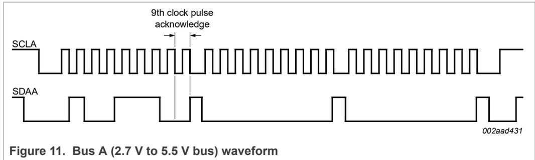
Figure 11. Bus A (2.7 V to 5.5 V bus) waveform
