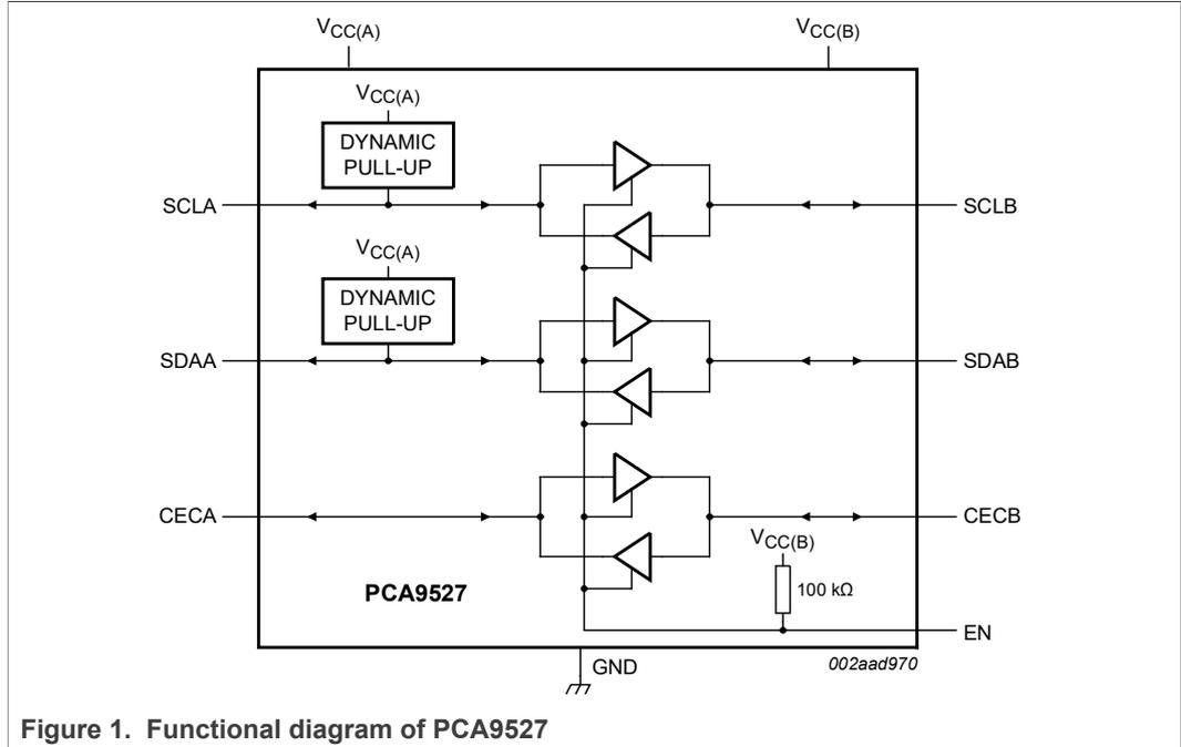
Figure 1. Functional diagram of PCA9527
