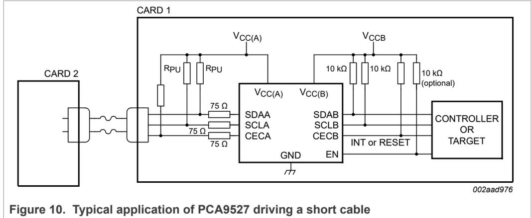
Figure 10. Typical application of PCA9527 driving a short cable
