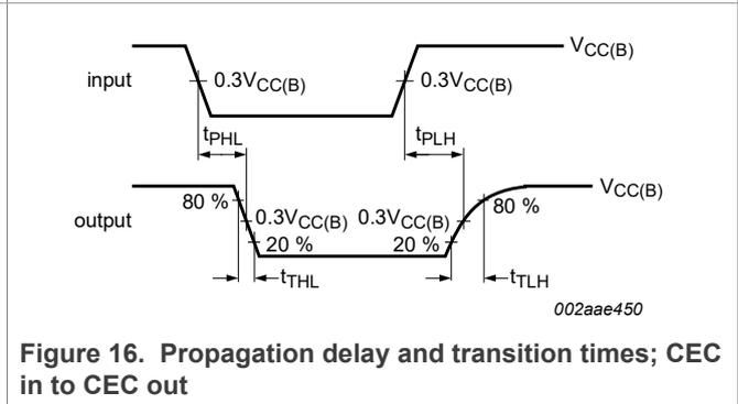
Figure 16. Propagation delay and transition times; CEC in to CEC out
