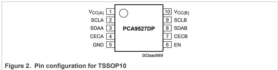
Figure 2. Pin configuration for TSSOP10
