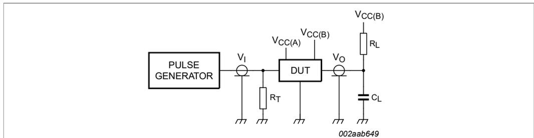
$R_L$  = load resistor; 1.35 k $\Omega$  on port B (2.7 V to 5 V) and 1.5 k $\Omega$  on port A (5.0 V).
