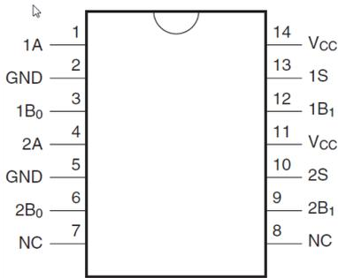
Figure 2. Pin Assignments for TSSOP (Top View)
