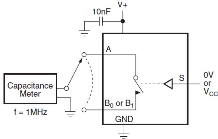
**Figure 10. On / Off Capacitance Measurement Setup**
