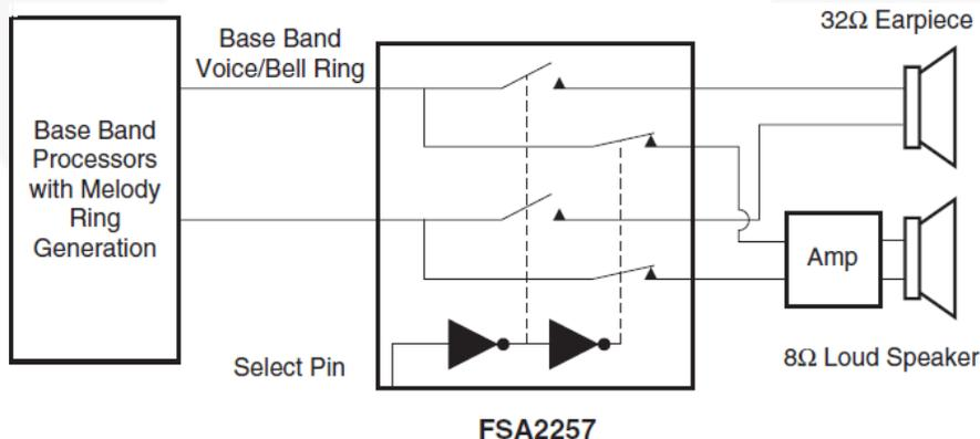
Figure 1. Block Diagram
