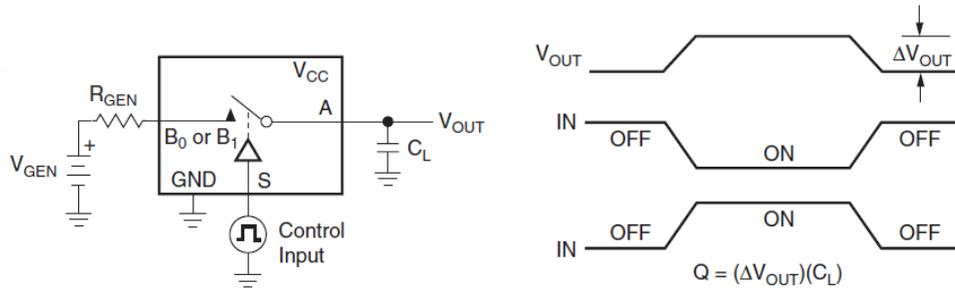
**Figure 9. Charge Injection**
