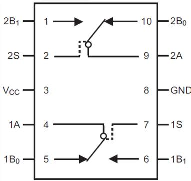
Figure 4. Pin Assignments for MSOP (Top View)
