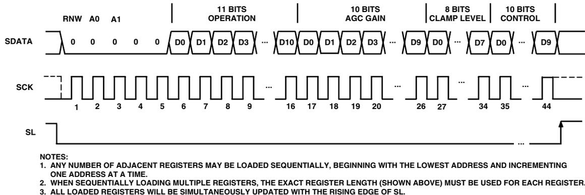
Figure 10. Continuous Serial Write Operation to Multiple Registers
