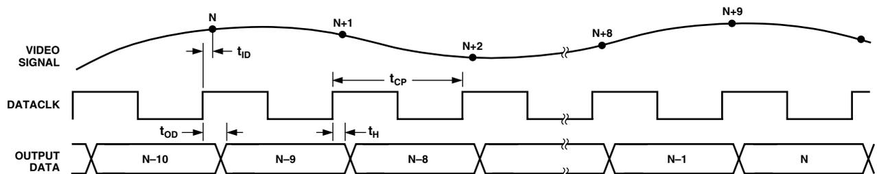
Figure 7. AUX-Mode Timing
