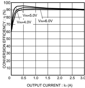
Fig.13 Conversion efficiency
