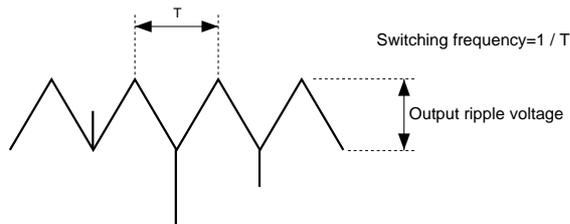
Note that the output ripple voltage depends on the type and characteristics of the output capacitor.
