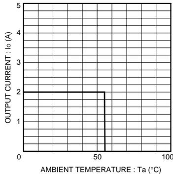
Fig.6 Derating curve
