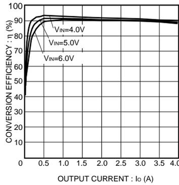
Fig.16 Conversion efficiency
