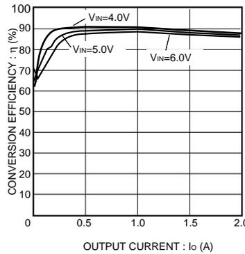
Fig.7 Conversion efficiency
