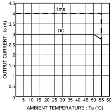
Fig.15 Derating curve
