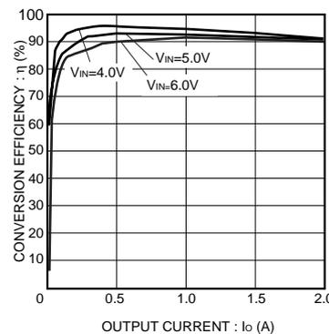
Fig.10 Conversion efficiency
