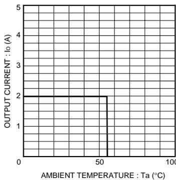
Fig.9 Derating curve
