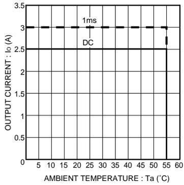
Fig.12 Derating curve
