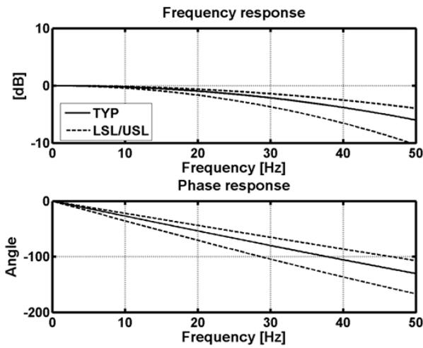
**Figure 3** Frequency response of SCA3000-E01 in measurement mode
