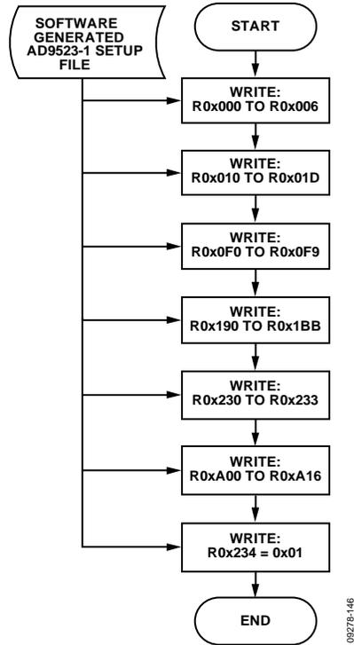
Figure 47. Subprocess: Write Registers from Setup File
