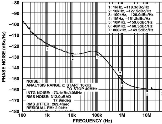
Figure 14. Phase Noise, Output = 184.32 MHz
