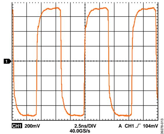
Figure 11. Output Waveform (Differential), LVPECL at 122.88 MHz
