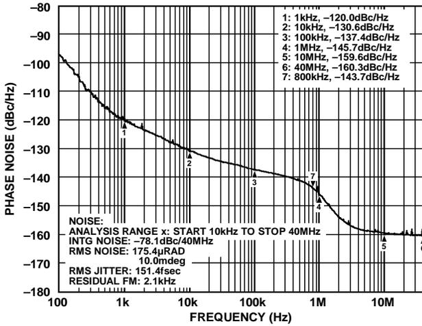
Figure 13. Phase Noise, Output = 184.32 MHz
