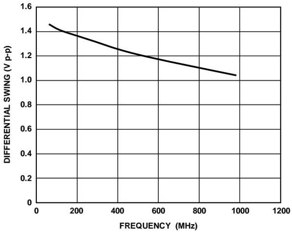
Figure 8. Differential Voltage Swing vs. Frequency, LVPECL Mode
