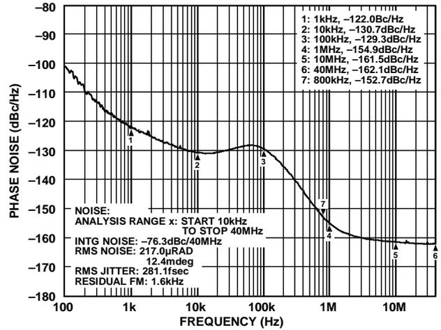
Figure 16. Phase Noise, Output = 122.88 MHz
