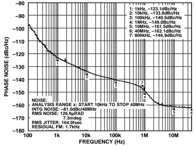
Figure 15. Phase Noise, Output = 122.88 MHz
