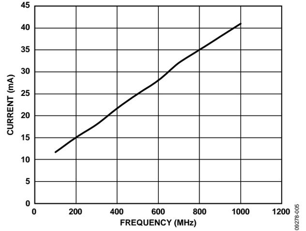
Figure 5. VDD3\_OUT[x;y] Current (Typical) vs. Frequency, LVPECL Mode
