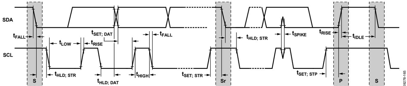
Figure 37. I<sup>2</sup>C Serial Port Timing
