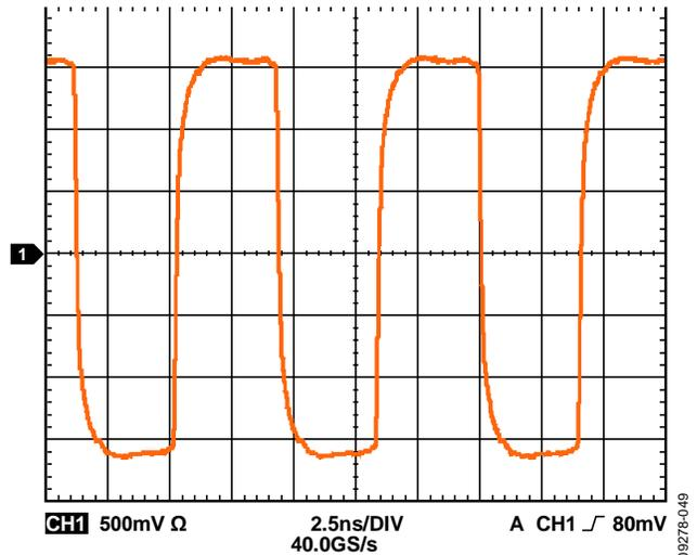
Figure 12. Output Waveform (Differential), HSTL at 16 mA, 122.88 MHz
