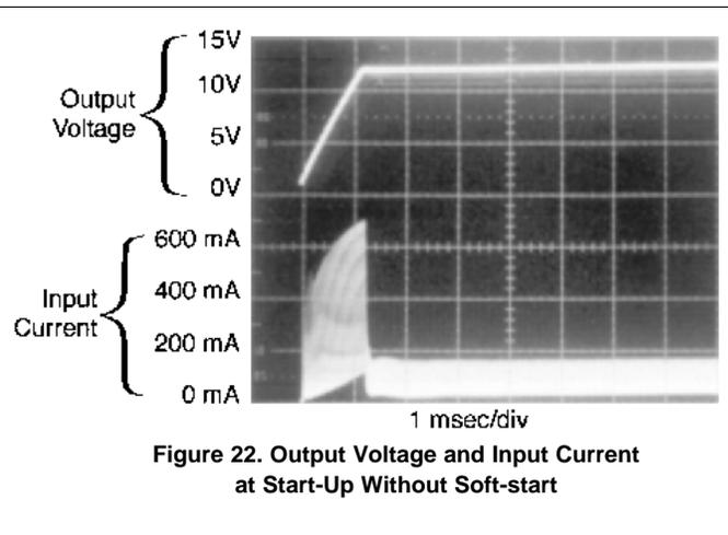
This reduction in start-up current is useful in situations where the input power source is limited in the amount of current it can deliver. In some applications, soft start can be used to replace undervoltage lockout or delayed start-up functions.
