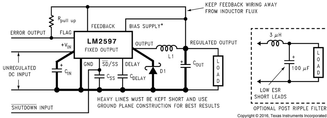
Component values shown are for  $V_{IN} = 15\text{ V}$ ,  $V_{OUT} = 5\text{ V}$ ,  $I_{LOAD} = 500\text{ mA}$
