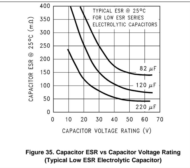
The consequences of operating an electrolytic capacitor above the RMS current rating is a shortened operating life. The higher temperature speeds up the evaporation of the electrolyte of the capacitor, resulting in eventual failure.
