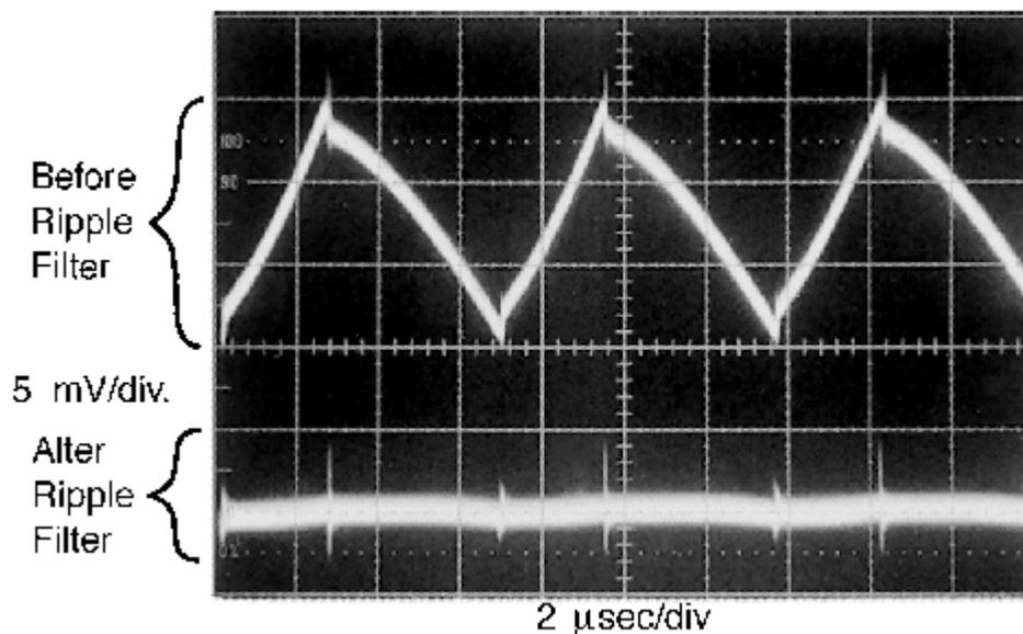
**Figure 30. Post Ripple Filter Waveform**
