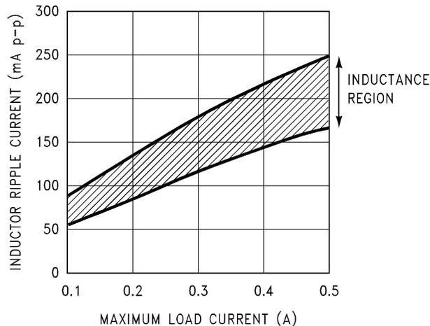
**Figure 42. Peak-to-Peak Inductor Ripple Current vs Load Current**
