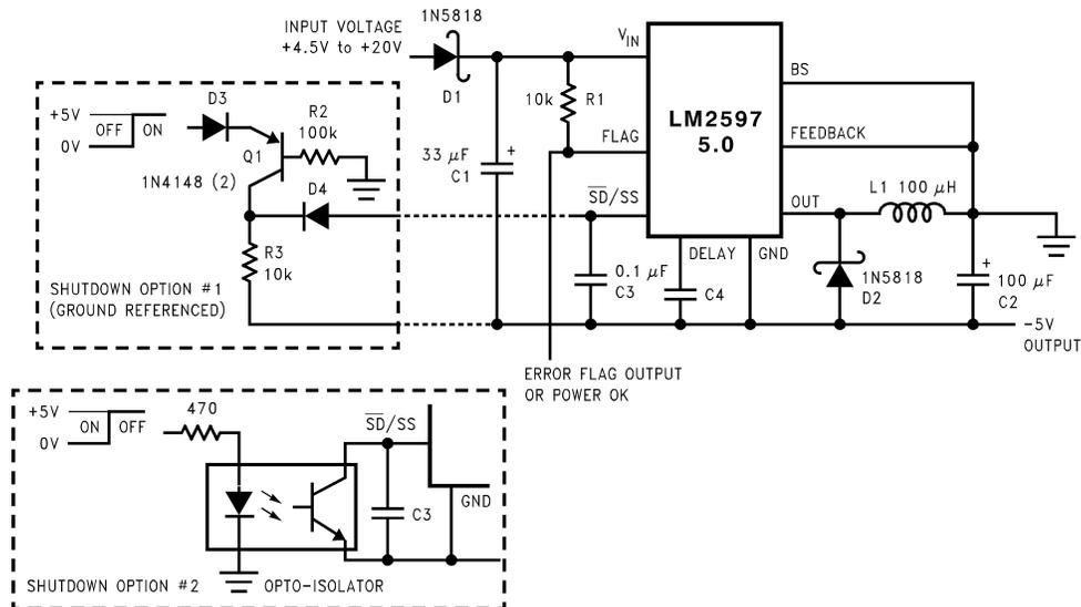
Figure 24. Inverting -5-V Regulator With Shutdown and Soft-Start
