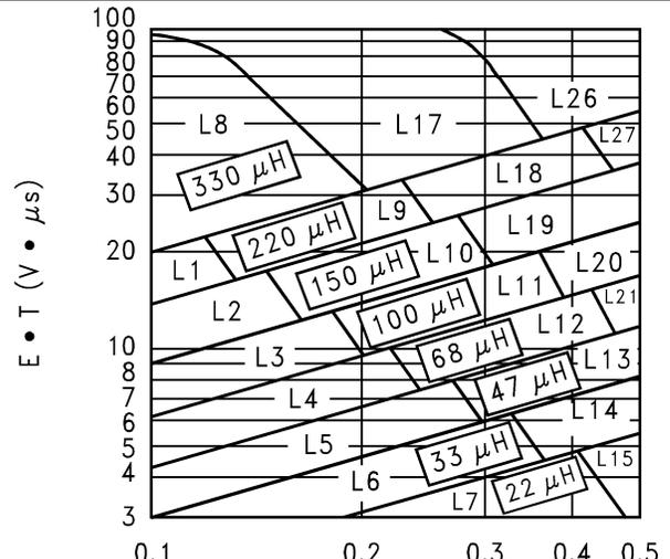
**Figure 41. LM2597xx Adjustable Voltage Version**
