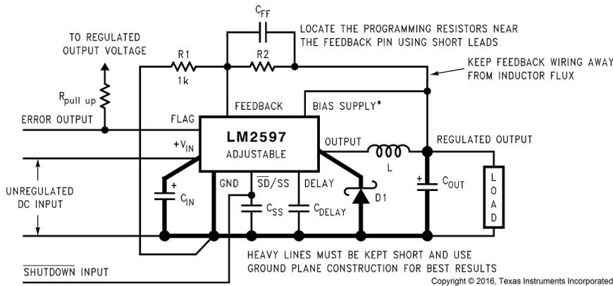
$$V_{OUT} = V_{REF} \left( 1 + \frac{R_2}{R_1} \right) \quad \text{where } V_{REF} = 1.23\text{V} \quad R_2 = R_1 \left( \frac{V_{OUT}}{V_{REF}} - 1 \right)$$
