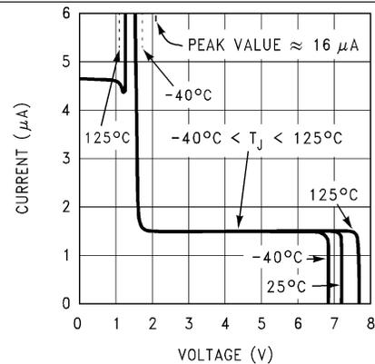
Figure 14. Shutdown/Soft-Start Current
