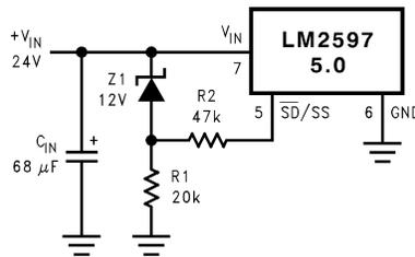
Figure 26. Undervoltage Lockout for a Buck Regulator
