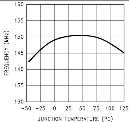
Figure 12. Switching Frequency
