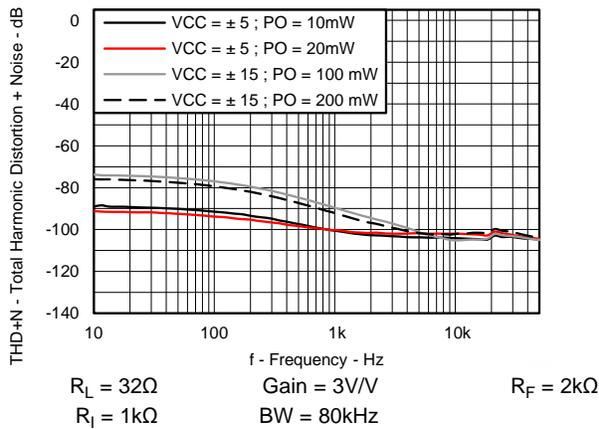
Figure 3. Total Harmonic Distortion + Noise versus Frequency
