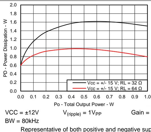
Figure 8. Power Dissipation versus Total Output Power
