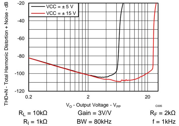
Figure 4. Total Harmonic Distortion + Noise versus Output Voltage
