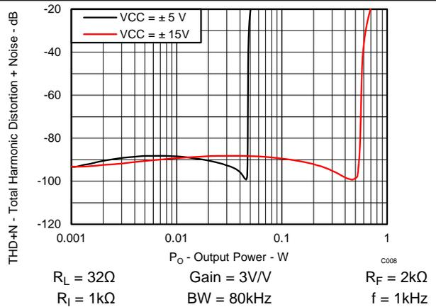
Figure 6. Total Harmonic distortion + Noise versus Output Power
