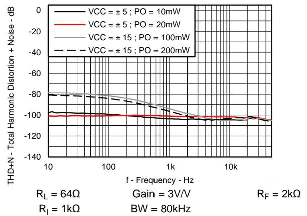
Figure 2. Total Harmonic Distortion + Noise versus Frequency
