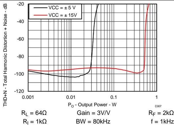
Figure 5. Total Harmonic Distortion + Noise versus Output Power
