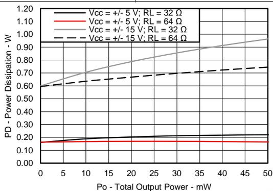
Figure 11. Power Dissipation versus Power Output - 50mW Scale
