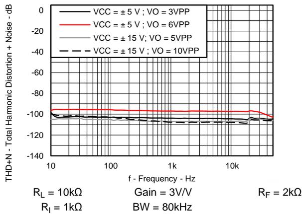
Figure 1. Total Harmonic Distortion + Noise versus Frequency
