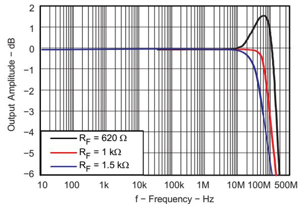
$$V_{CC} = \pm 5V \quad \text{Gain} = 1V/V \quad R_L = 25\Omega$$
