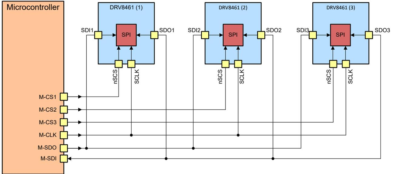
Figure 7-55. Three Devices Connected in Parallel Configuration
