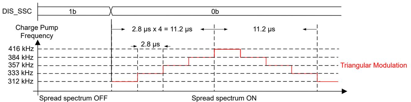
**Figure 7-38. Triangular Spread Spectrum of Charge Pump Clock**
