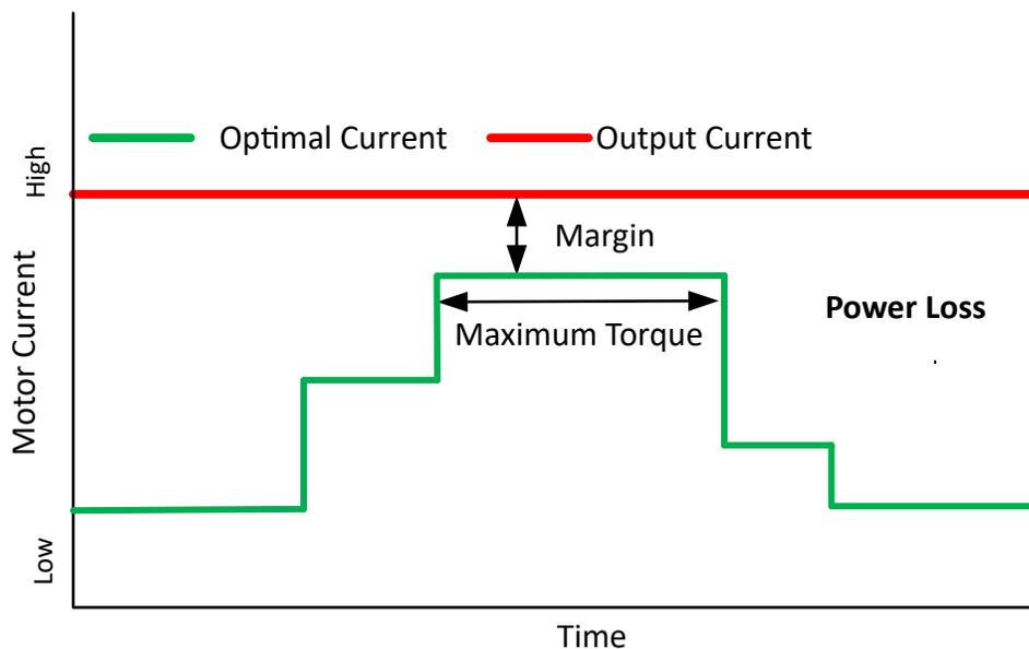
Figure 7-21. Power Loss with Conventional Stepper Driver
