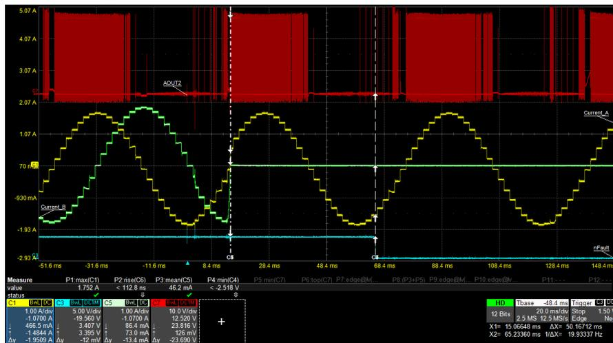
**Figure 7-45. Coil B open-load detection**
