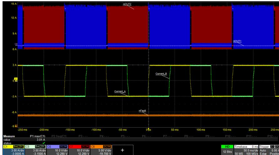
Figure 8-3. Full-step at 25 pps with  $I_{FS} = 3\text{ A}$
