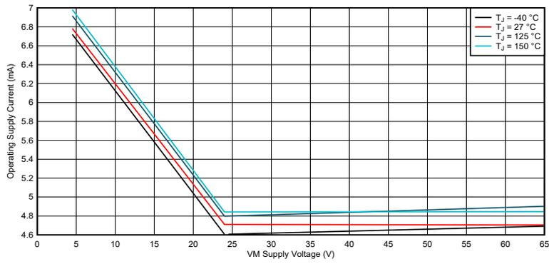
Figure 6-4. Operating supply current, VCC = External 5 V
