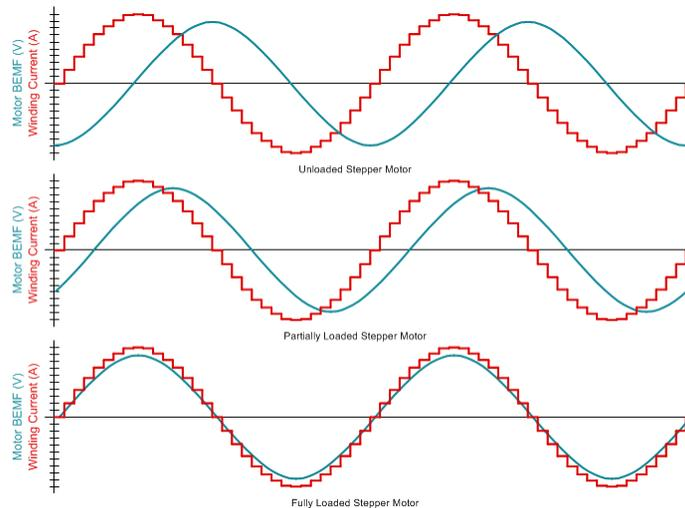
**Figure 7-42. Stall Detection by Monitoring Motor Back-EMF**
