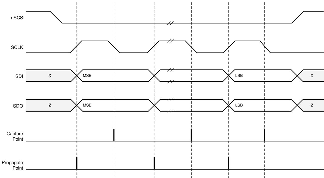
**Figure 7-54. SPI Transaction**
