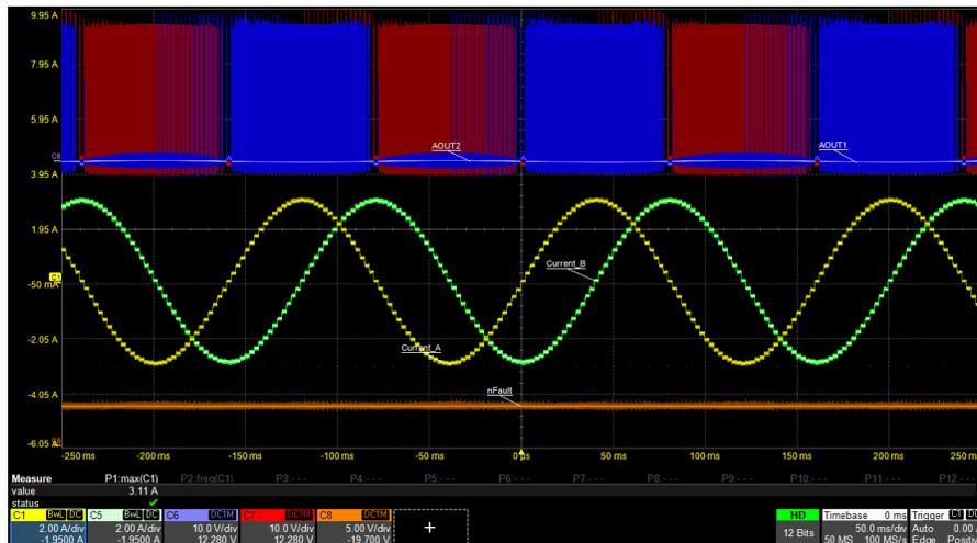
Figure 8-2. 1/16 microstepping at 400 pps with  $I_{\text{FS}} = 3 \text{ A}$
