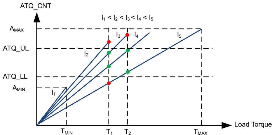
**Figure 7-26. ATQ\_CNT as a function of load torque**
