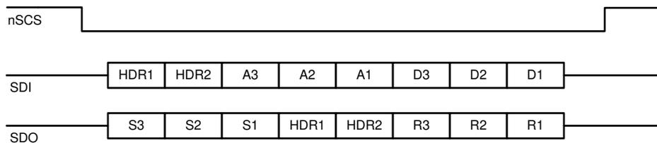
**Figure 7-51. SPI Data Sequence for Three Devices**
