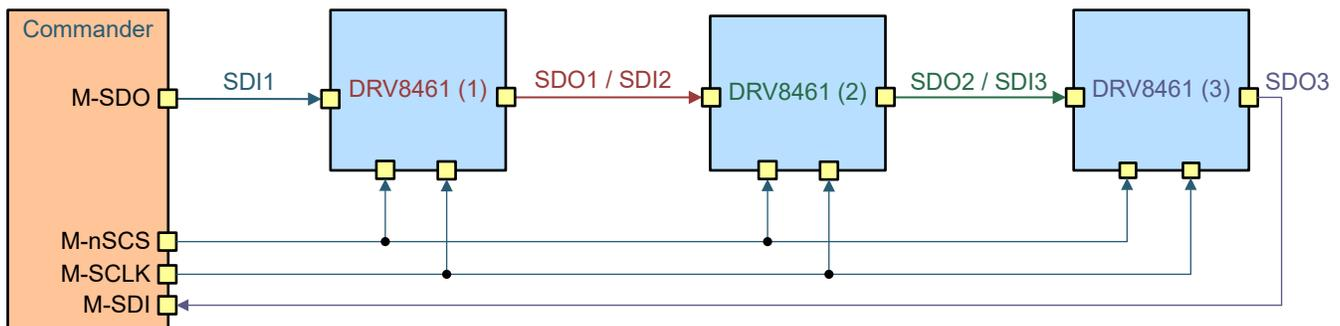
**Figure 7-49. Three Devices Connected in Daisy Chain**
