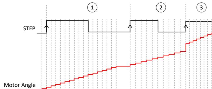
**Figure 7-8. Automatic Microstepping with Changing STEP Frequency**
