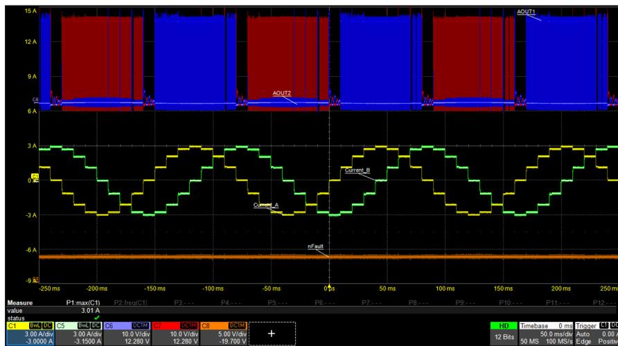
Figure 8-4. 1/4 microstepping at 100 pps with  $I_{FS} = 3\text{ A}$
