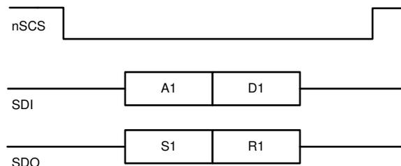
**Figure 7-48. SPI Format - Standard "16-bit" Frame**
