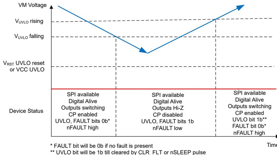
Figure 7-39. Supply Voltage Ramp Profile
