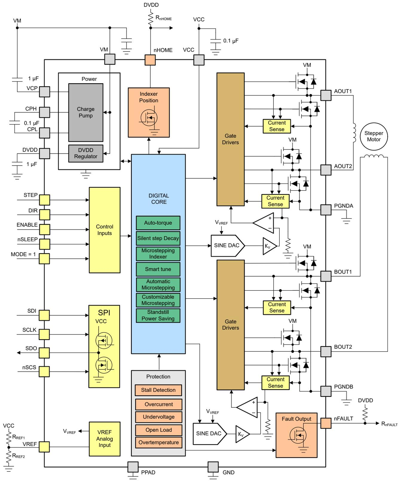
Figure 7-1. DRV8461 Block Diagram with SPI Interface
