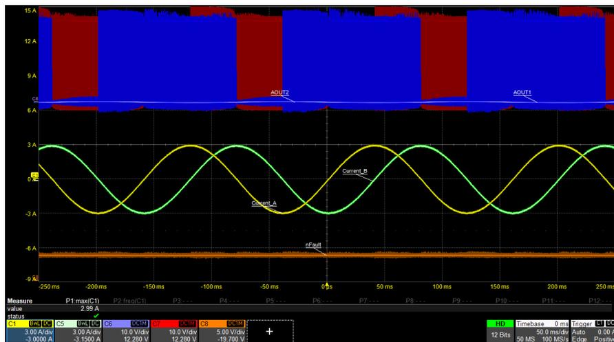
Figure 8-5. 1/256 microstepping at 6400 pps with  $I_{FS} = 3\text{ A}$
