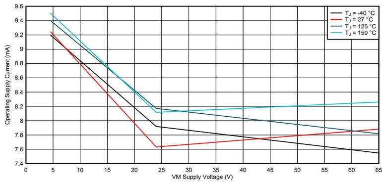
Figure 6-5. Operating supply current, VCC = DVDD
