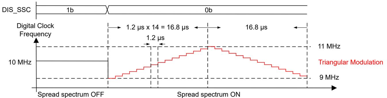
**Figure 7-37. Triangular Spread Spectrum of Internal Digital Clock**
