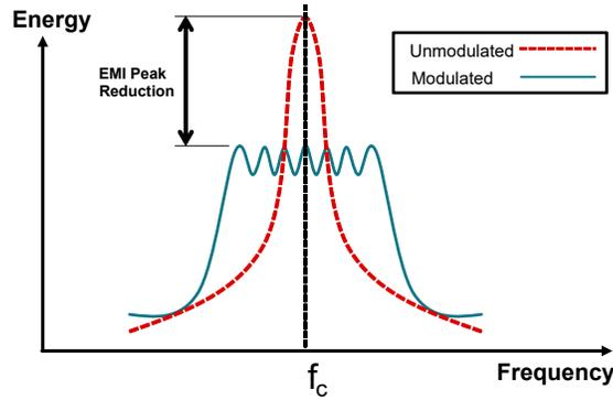
**Figure 7-36. EMI Reduction by Spread Spectrum, Frequency Modulation**
