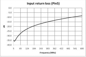
Electrical Specifications:  $Z_0 = 75\Omega$ ,  $T_A = 25$ °C,  $P_{in} = 0$ dBm
