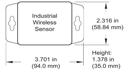
**ALTA Industrial Wireless Accelerometer - Advanced Vibration Meter (Leaded) | Technical Specifications**
