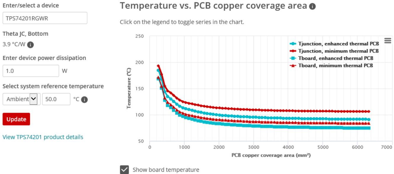
**Figure 13. TI PCB Thermal Calculator Example**
