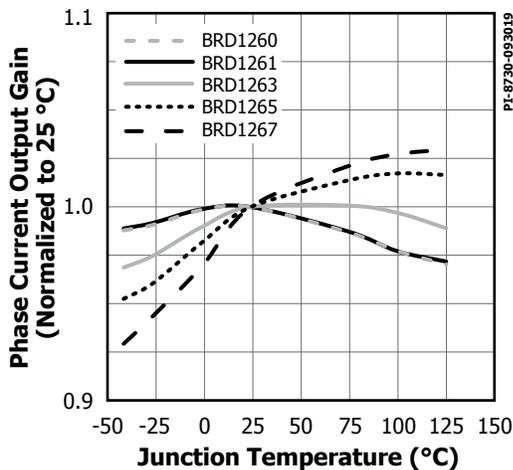
Figure 35. Phase Current Output Gain vs. Temperature
