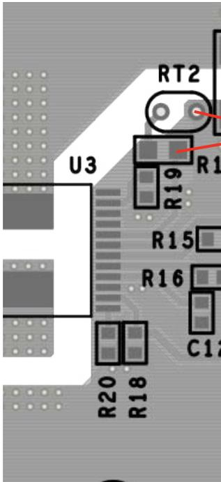
Thermistor and Series Resistor Configured as System Temperature Monitor
