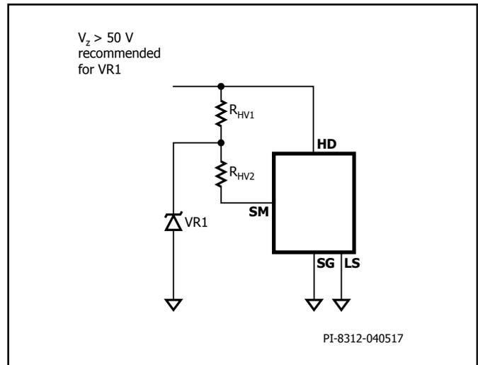
Figure 18. High-Voltage Bus Monitoring with Overvoltage Protection Disabled.
