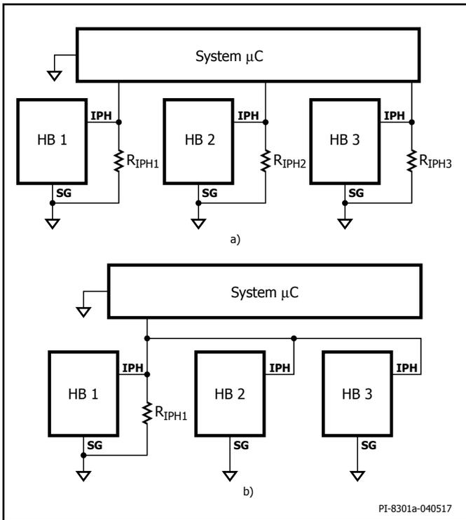
Figure 13. Phase Current Information through IPH Pin with BRD126X
