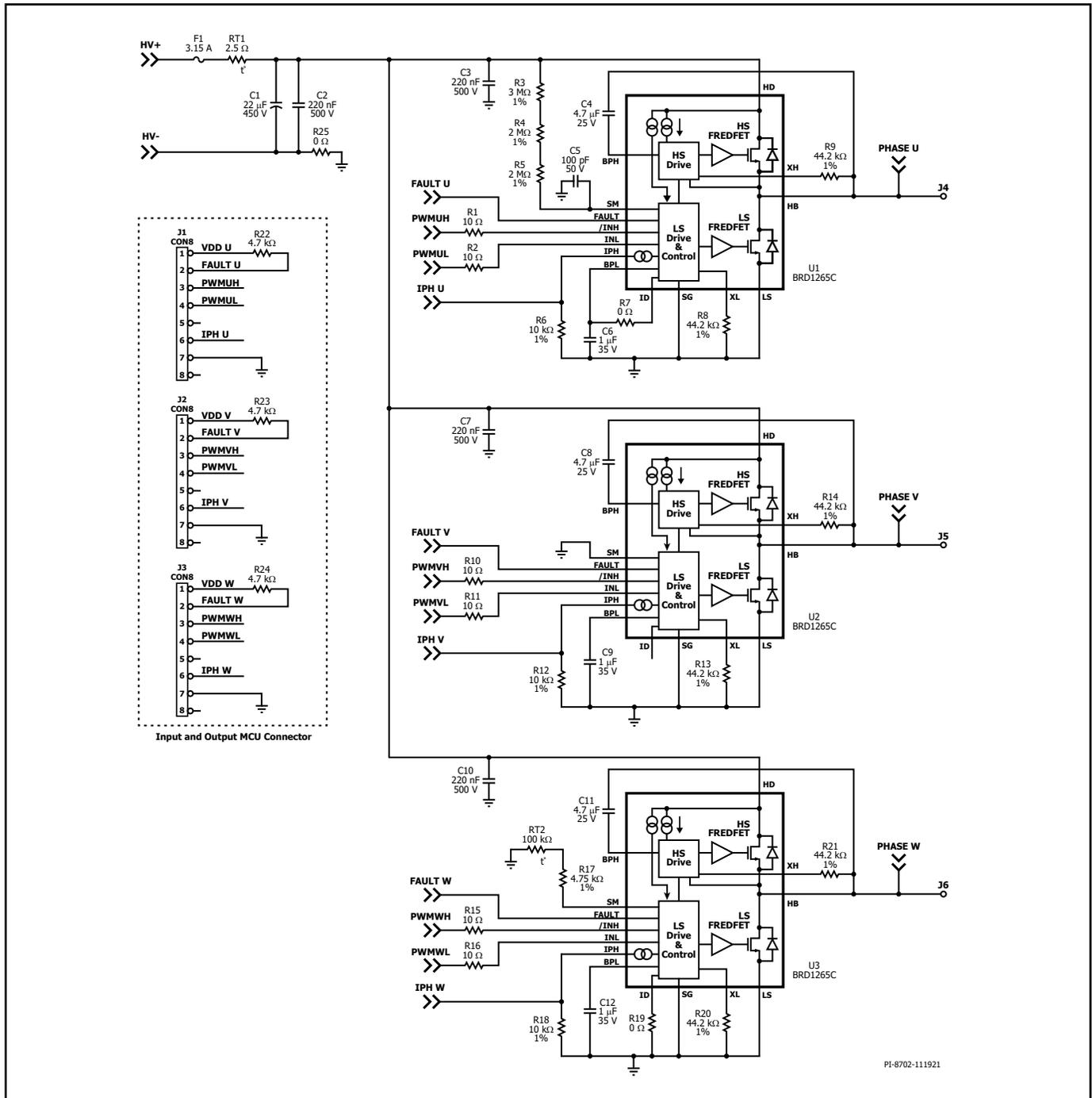
Figure 22. Schematic DER-654. Three-Phase Inverter Example using BRD1265C.
