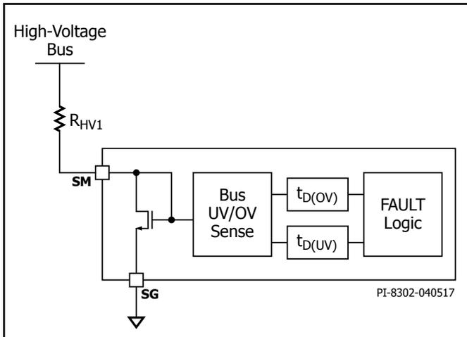
Figure 15. High-Voltage Bus Monitoring with SYSTEM MONITOR Pin.
