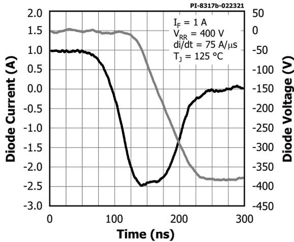
Figure 31. Typical Diode Reverse Recovery (BRD1X67).
