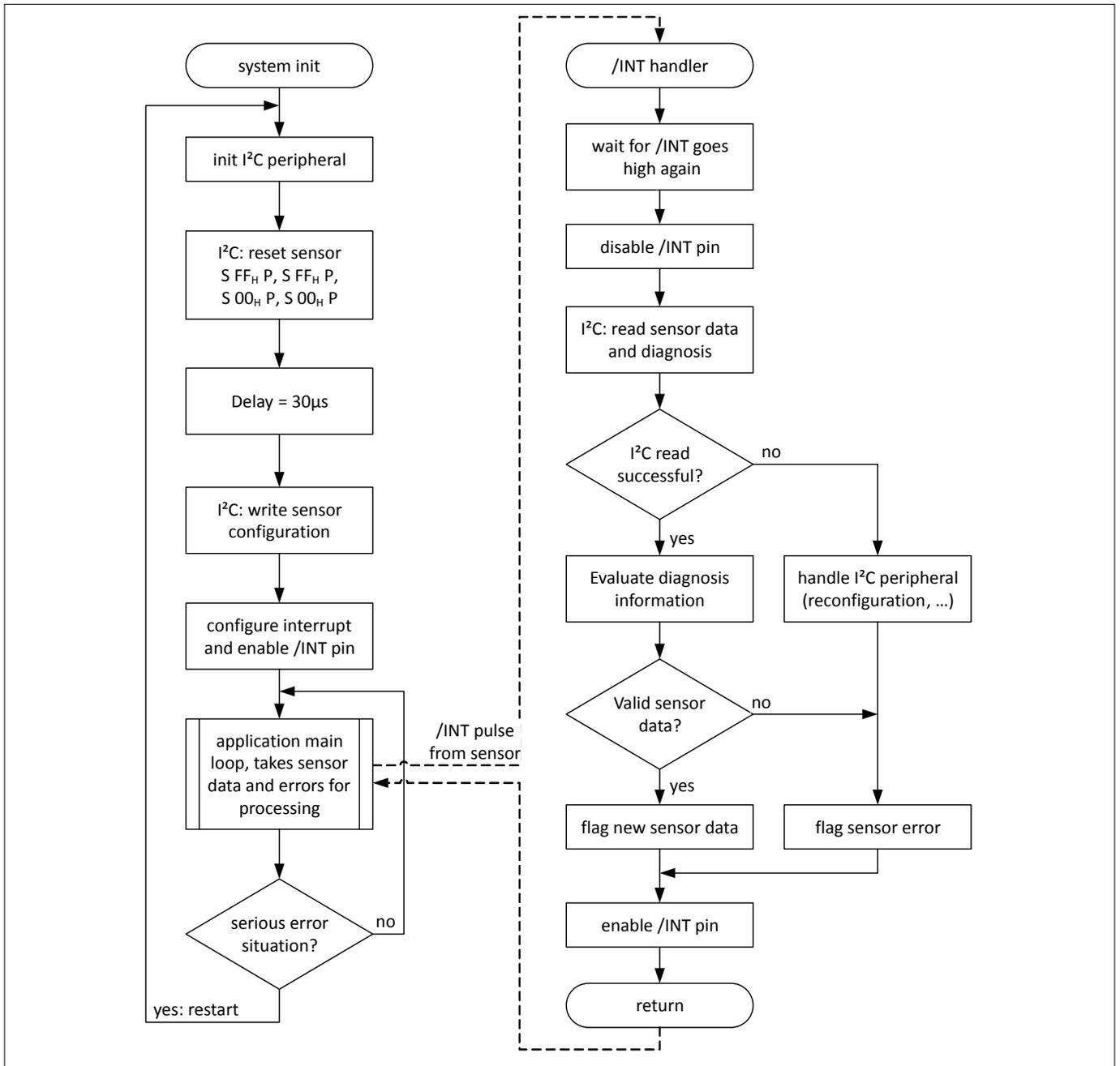
Figure 13 Microcontroller software flowchart for TLE493D-P2B6
