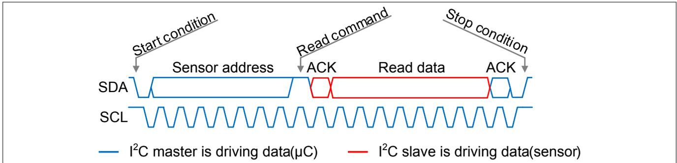
**Figure 8** General I<sup>2</sup>C frame format 1-byte: Read data from sensor to microcontroller
