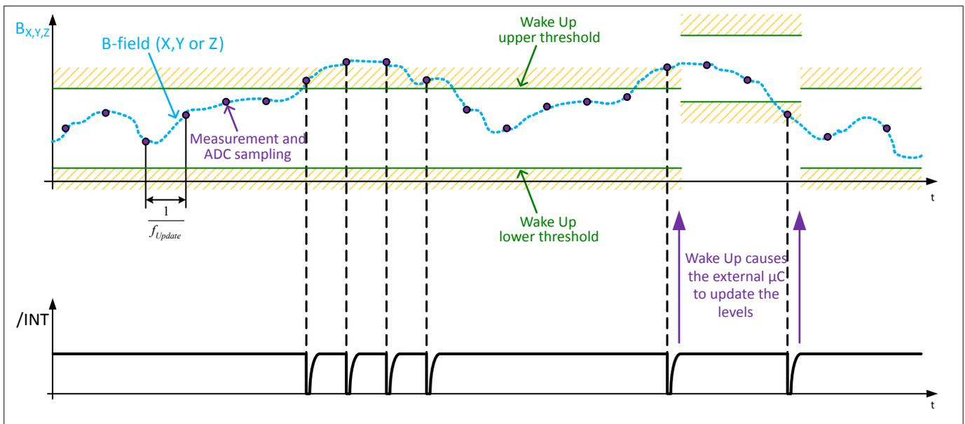
**Figure 15** Static or Dynamic Wake Up Threshold Operation of the TLE493D-P2B6
