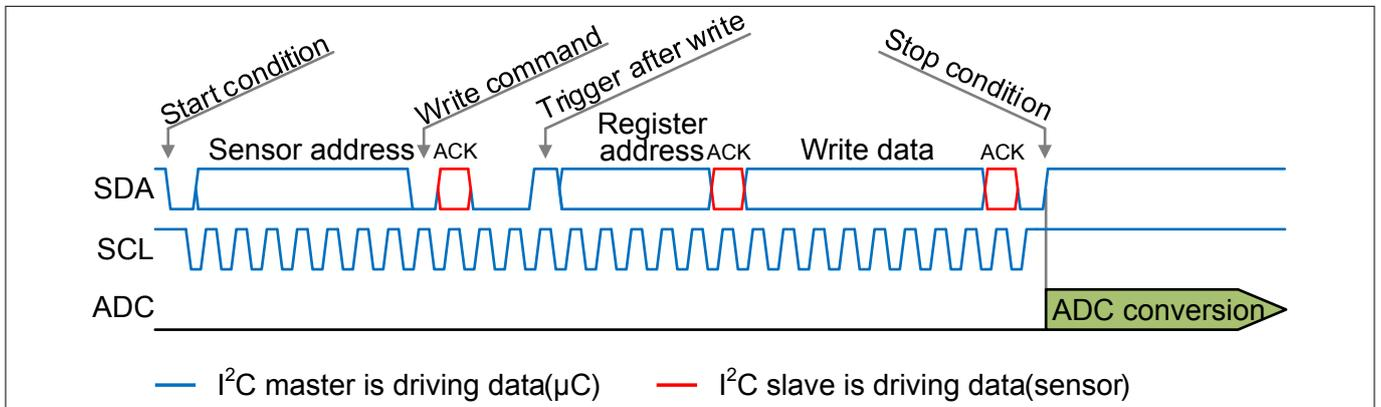
**Figure 4** ADC trigger after write frame is finished, I<sup>2</sup>C trigger bits 001<sub>B</sub>
