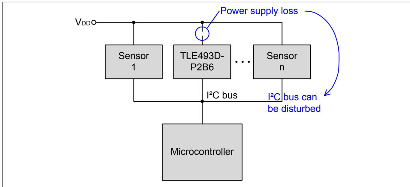
**Figure 14** Example of I<sup>2</sup>C bus and a TLE493D-P2B6 with disconnected V<sub>DD</sub>
