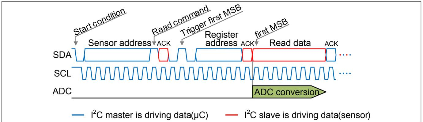
**Figure 3** ADC trigger before sending first MSB of data registers, I<sup>2</sup>C trigger bits 010<sub>B</sub>
