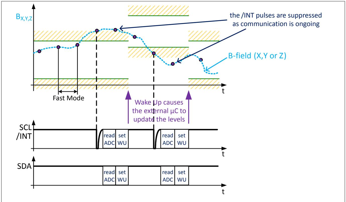
**Figure 16** Dynamic Wake Up Threshold Operation of the TLE493D-P2B6 for Bandwidth Reduction
