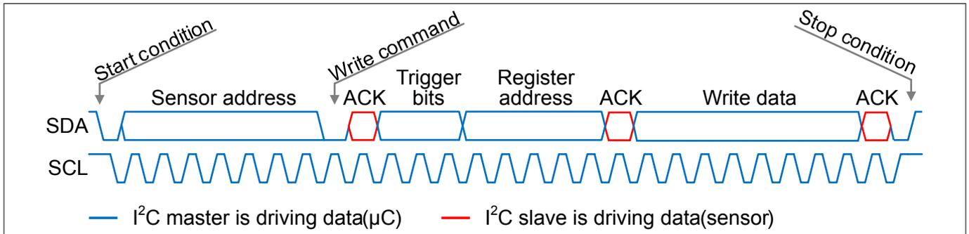
**Figure 2** General I<sup>2</sup>C write frame format: Write data from microcontroller to sensor
