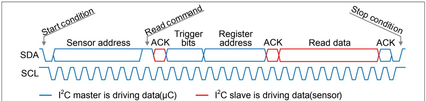
**Figure 7 General I<sup>2</sup>C frame format 2-byte: Read data from sensor to microcontroller**
