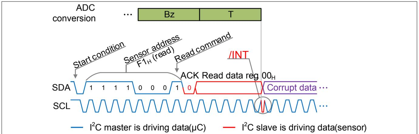
**Figure 10** Example without collision avoidance CA bit = 1<sub>B</sub> and INT bit = 0<sub>B</sub>
