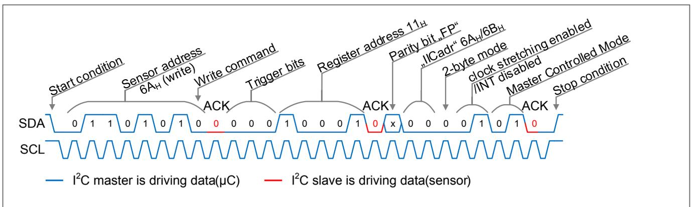
**Figure 6 Example I<sup>2</sup>C frame format 2-byte: Write data from microcontroller to sensor**
