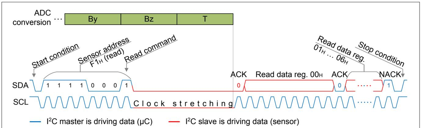
**Figure 12** Example with clock stretching CA bit = 0<sub>B</sub> and INT bit = 1<sub>B</sub>
