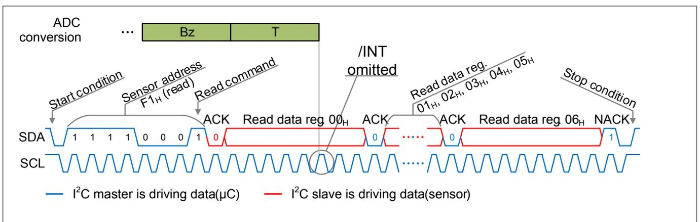
**Figure 11** Example with collision avoidance CA bit = 0<sub>B</sub> and INT bit = 0<sub>B</sub>
