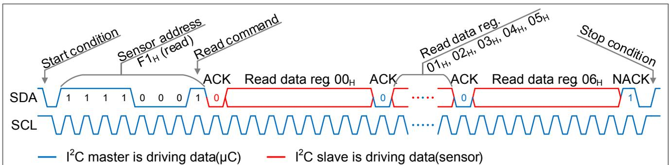
**Figure 9** Example I<sup>2</sup>C frame format 1-byte: Read data from sensor to microcontroller
