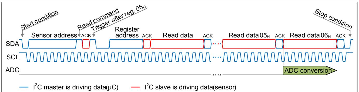
**Figure 5** ADC trigger after register 05<sub>H</sub>, I<sup>2</sup>C trigger bits 100<sub>B</sub>
