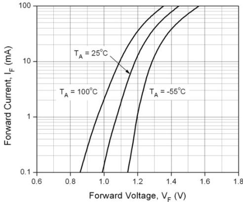
Figure 2. Transfer Characteristics
