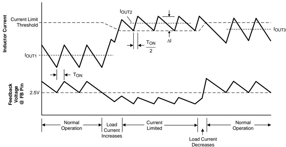
Figure 10. Inductor Current - Normal and Current Limit Operation
