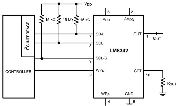
Figure 27. Programmable Current Sink
