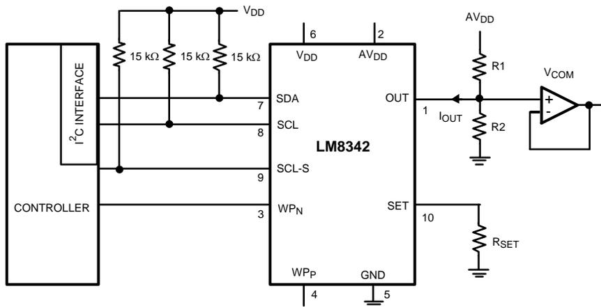
Figure 28. Typical Application Driving a  $V_{COM}$  Level
