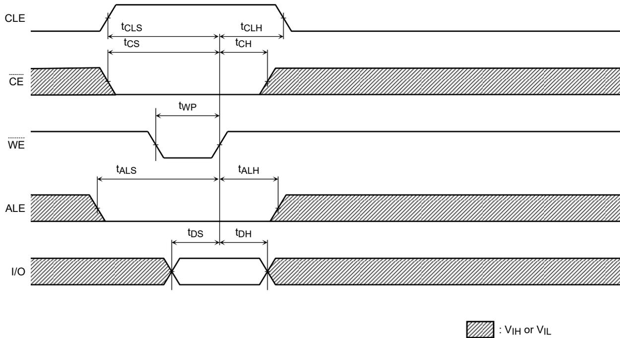
Address Input Cycle Timing Diagram
