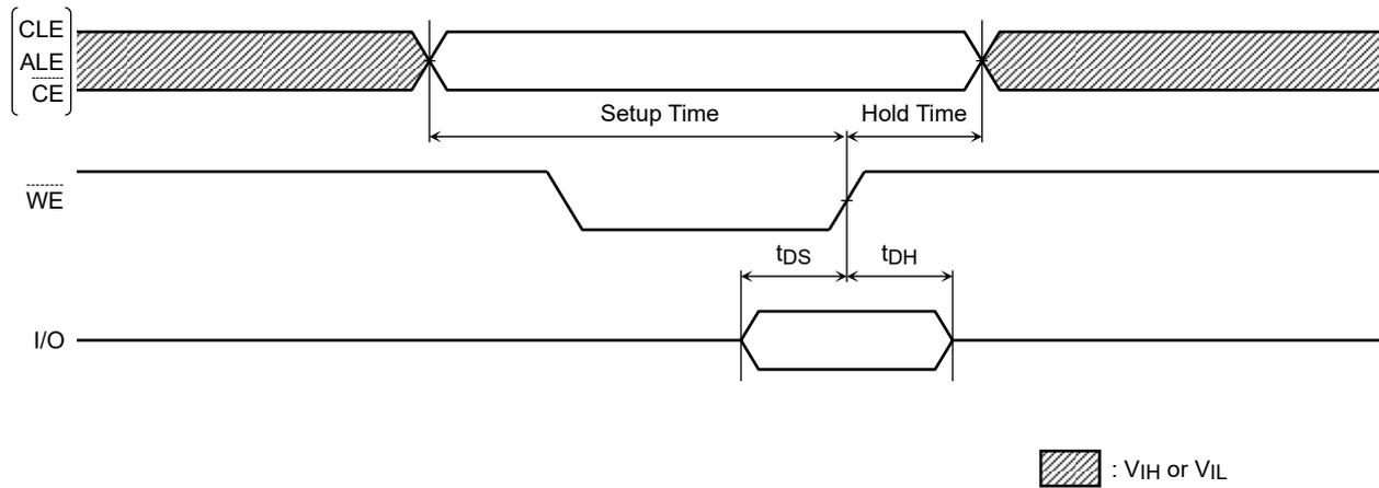
Command Input Cycle Timing Diagram
