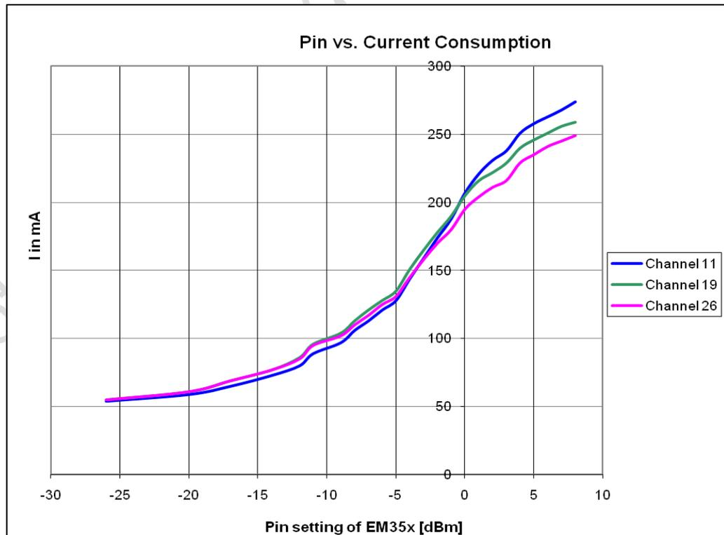
**Figure 4. Module Current vs. Power Setting**
