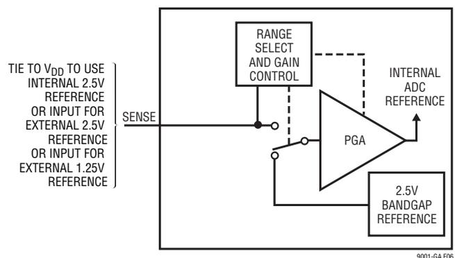
**Figure 6. Reference Circuit**
