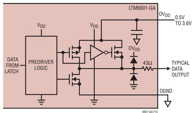
Figure 9. Equivalent Circuit for a Digital Output Buffer
