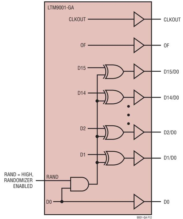
**Figure 10. Functional Equivalent of Digital Output Randomizer**
