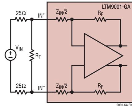
**Figure 2. Input Termination for Differential 50Ω Input Impedance Using Shunt Resistor (See Table 2 for R<sub>T</sub> Values)**
