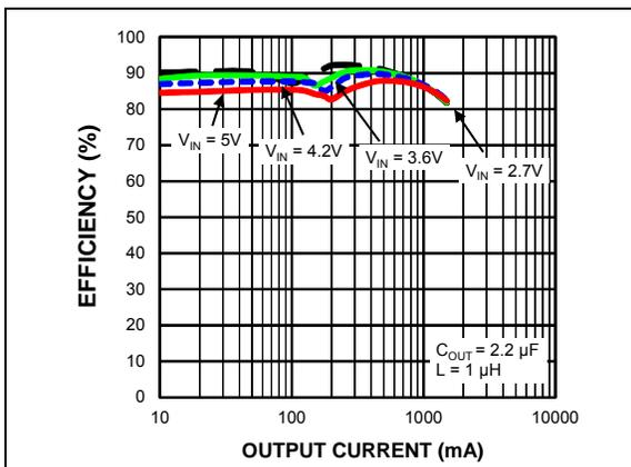
**FIGURE 2-2:** Efficiency ( $V_{OUT} = 1.8V$ ) vs. Output Current.
