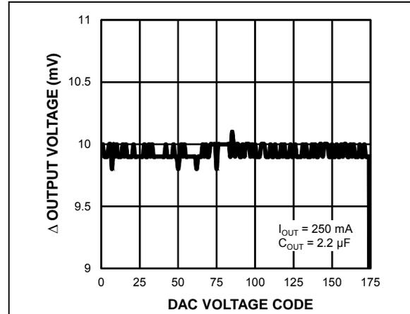
**FIGURE 2-16:**  $\Delta$  Output Voltage vs. DAC DNL.
