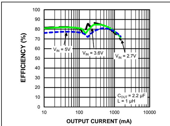
**FIGURE 2-3:** Efficiency ( $V_{OUT} = 1.0V$ ) vs. Output Current.
