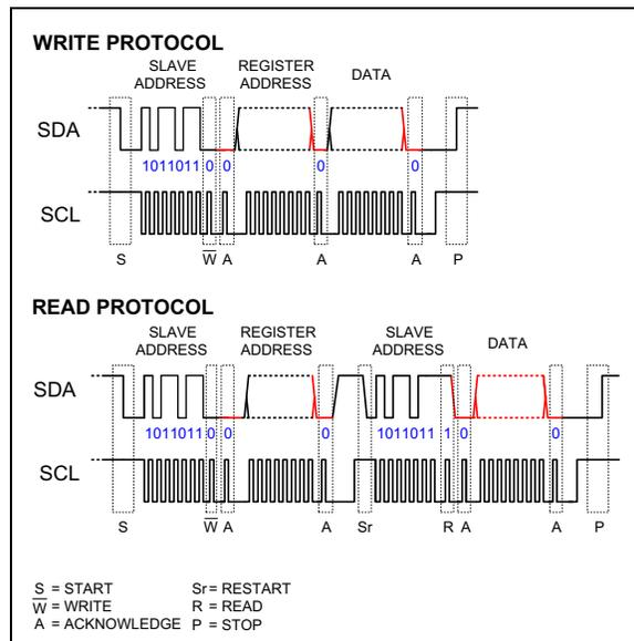
**FIGURE 5-4:** Required Communications for Read/Write Operations via I<sup>2</sup>C Interface.
