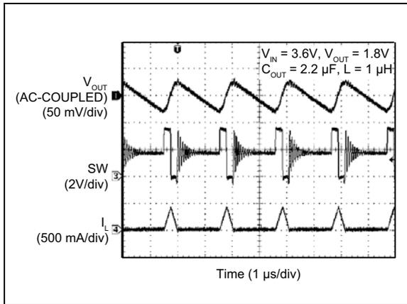
**FIGURE 2-20:** Switching Waveform Discontinuous Mode (50 mA).
