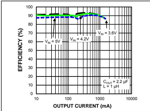
**FIGURE 2-1:** Efficiency ( $V_{OUT} = 2.4V$ ) vs. Output Current.
