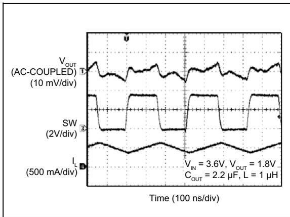
**FIGURE 2-21:** Switching Waveform Continuous Mode (500 mA).
