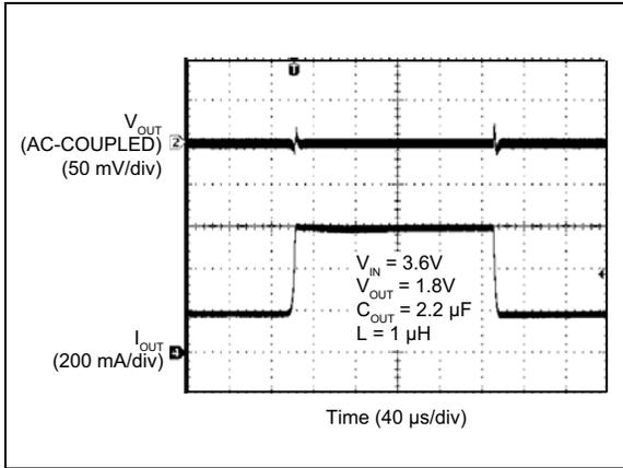
**FIGURE 2-25:** Load Transient (200 mA to 600 mA).
