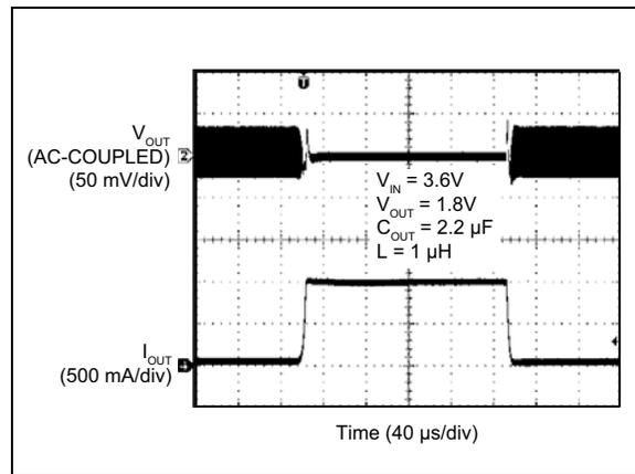
**FIGURE 2-24:** Load Transient (50 mA to 1A).
