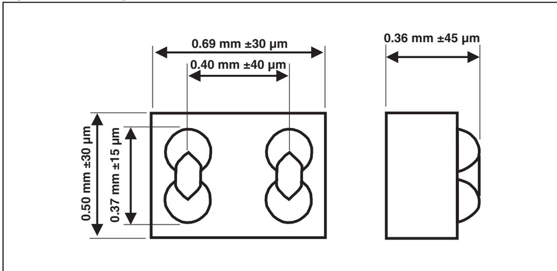
Figure 13. Flip Chip tape and reel specification
