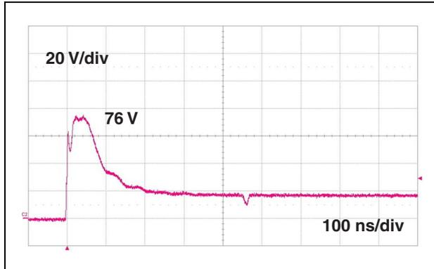
Figure 10. ESD response to IEC61000-4-2 (-15 kV air discharge)
