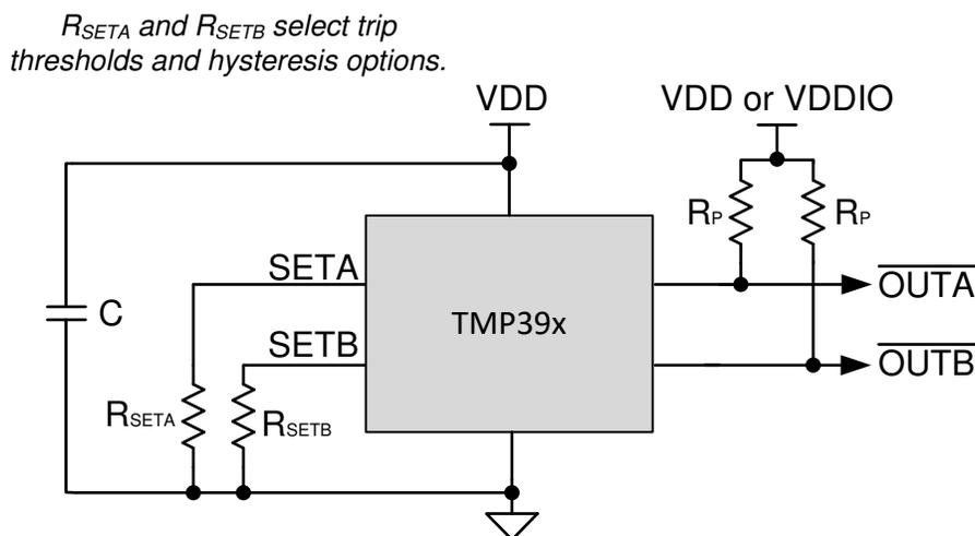
**Figure 7. Simplified Schematic**
