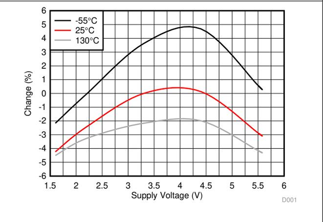
Figure 4. Sampling Period Variation vs Supply Voltage
