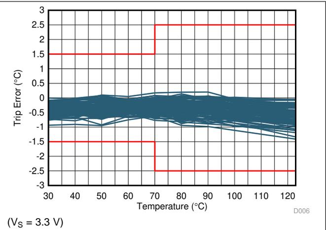
Figure 2. Hot Trip Point Accuracy vs Operating Temperature
