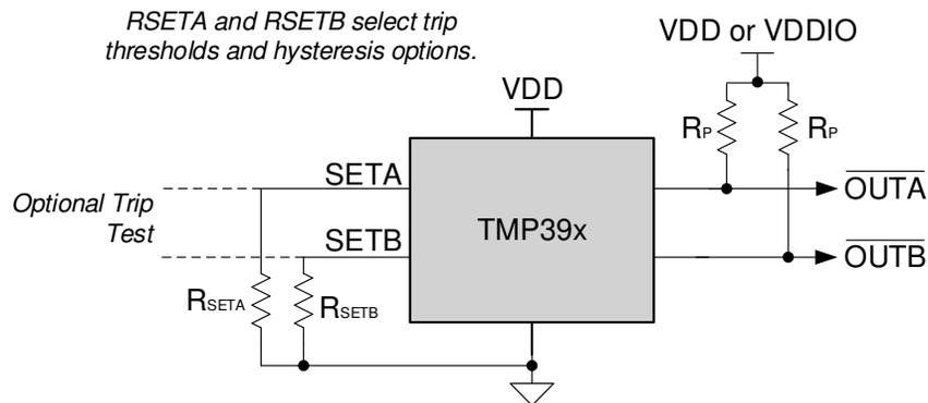
Figure 9. Simplified Schematic
