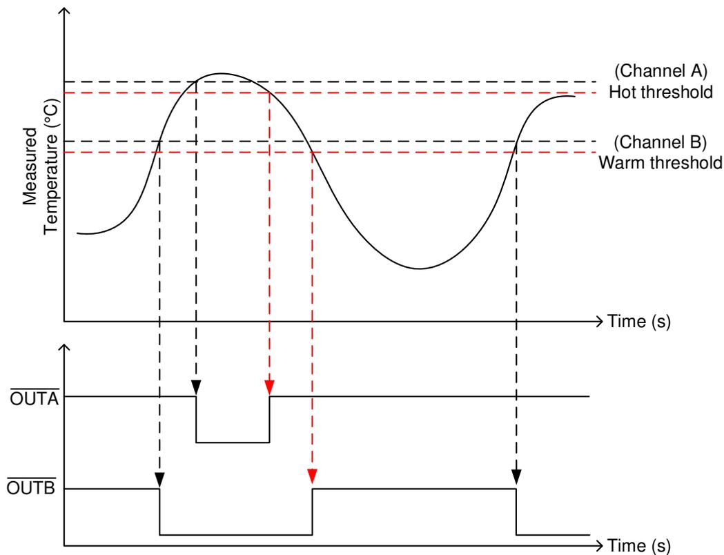
Figure 10. TMP392 Output With Hot/Warm Thresholds and Hysteresis
