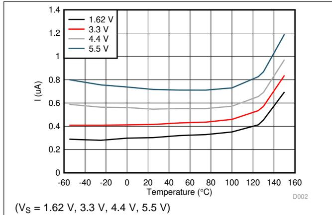
Figure 1. Average Supply Current vs Operating Temperature
