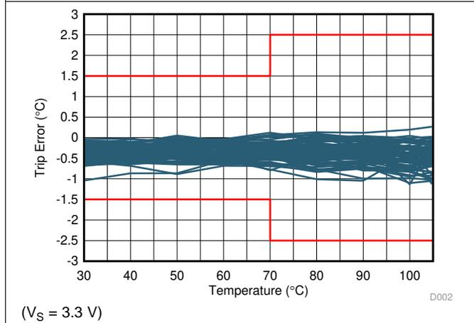
Figure 3. Warm Trip Point Accuracy vs Operating Temperature
