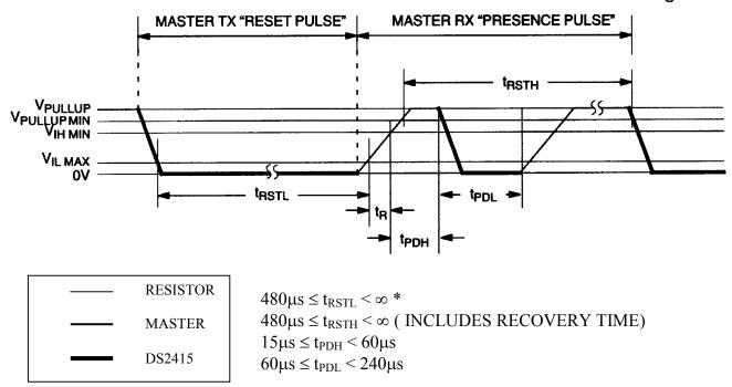
\* In order not to mask interrupt signaling by other devices on the 1-Wire bus,  $t_{RSTL} + t_R$  should always be less than 960 $\mu$ s.
