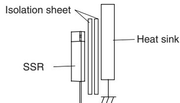
Please keep 5mm distance as minimum between naked metal portion of SSR and heat sink, and also between naked metal portion of SSR and bis/nut/washer.
