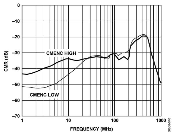
Figure 31. Common-Mode Rejection
