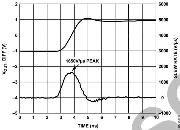
Figure 27. Large Signal Rising Edge Slew Rate
