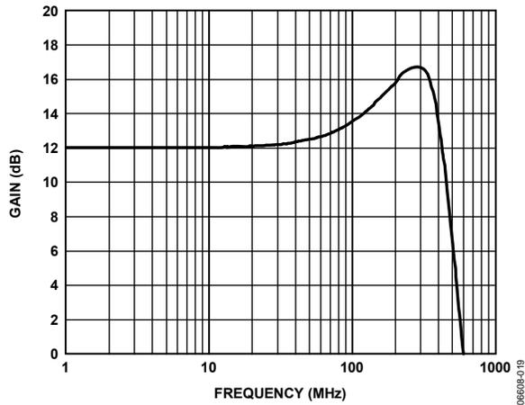
Figure 20. Small Signal Frequency Response, 200 mV p-p
