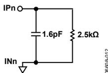
Figure 12. Receiver Simplified Equivalent Circuit When Driving Single-Ended
