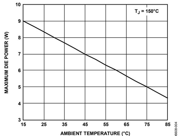
Figure 4. Maximum Die Power Dissipation vs. Ambient Temperature
