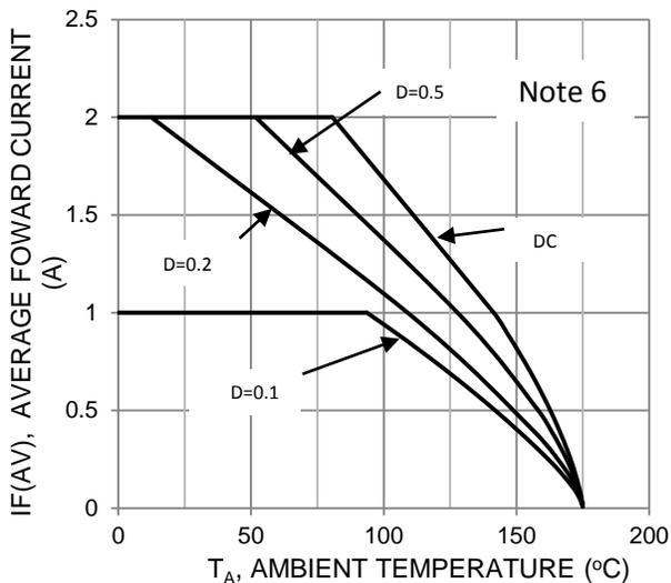
Figure 5 Forward Current Derating
