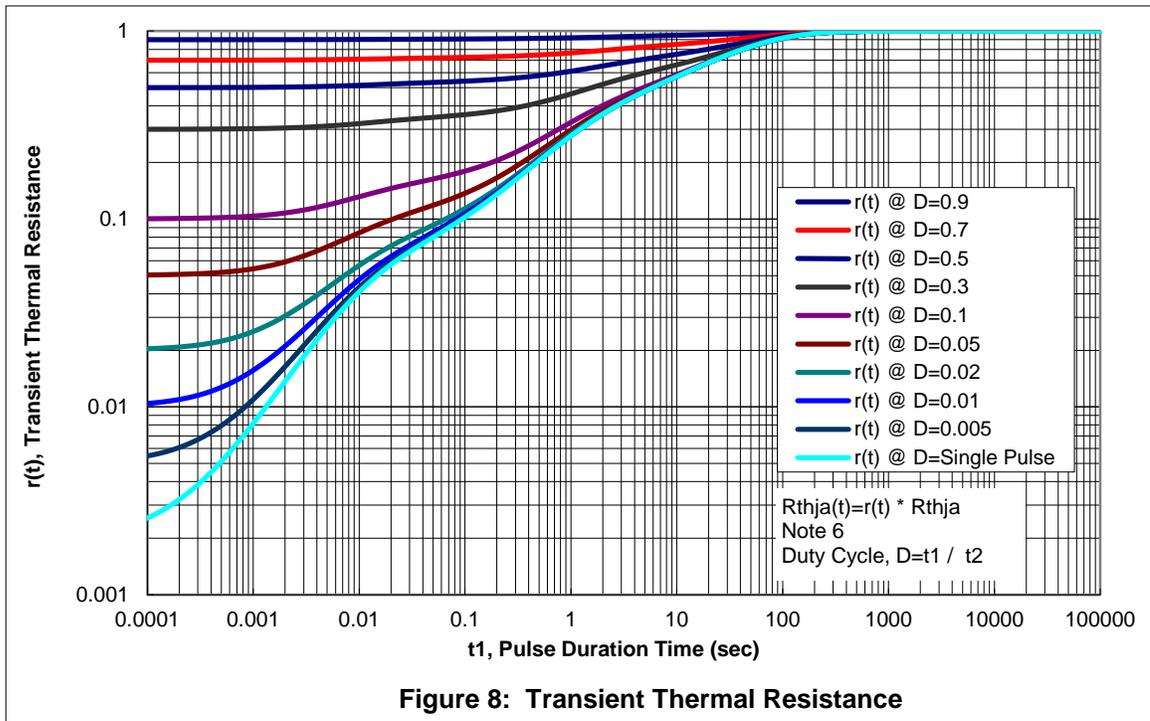
Figure 8: Transient Thermal Resistance
