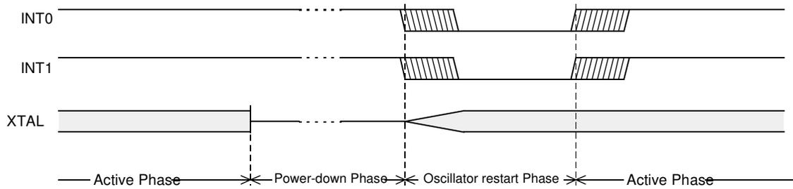
Exit from power-down by reset redefines all the SFRs, exit from power-down by external interrupt does not affect the SFRs.
