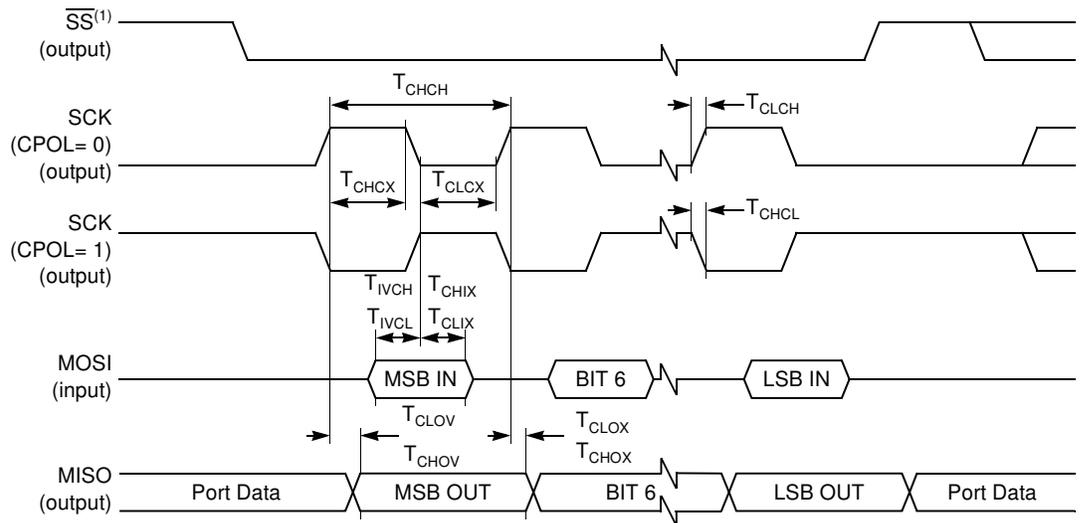
$\overline{SS}$  handled by software using general purpose port pin.
