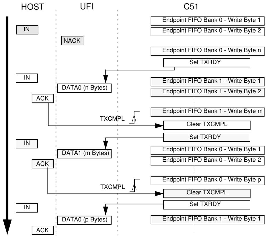
An endpoint will be first enabled and configured before being able to send Bulk or Interrupt packets.
