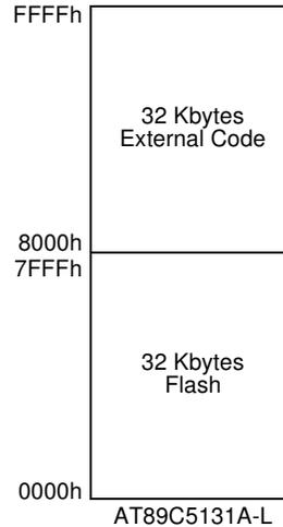
Note: If the program executes exclusively from on-chip code memory (not from external memory), beware of executing code from the upper byte of on-chip memory (7FFFh) and thereby disrupting I/O Ports 0 and 2 due to external prefetch. Fetching code constant from this location does not affect Ports 0 and 2.
