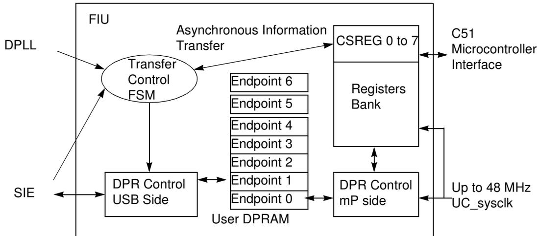
**Figure 59.** Minimum Intervention from the USB Device Firmware
