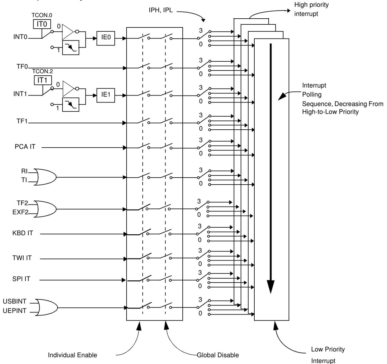
Each of the interrupt sources can be individually enabled or disabled by setting or clearing a bit in the Interrupt Enable register (Table 61). This register also contains a global disable bit, which must be cleared to disable all interrupts at once.
