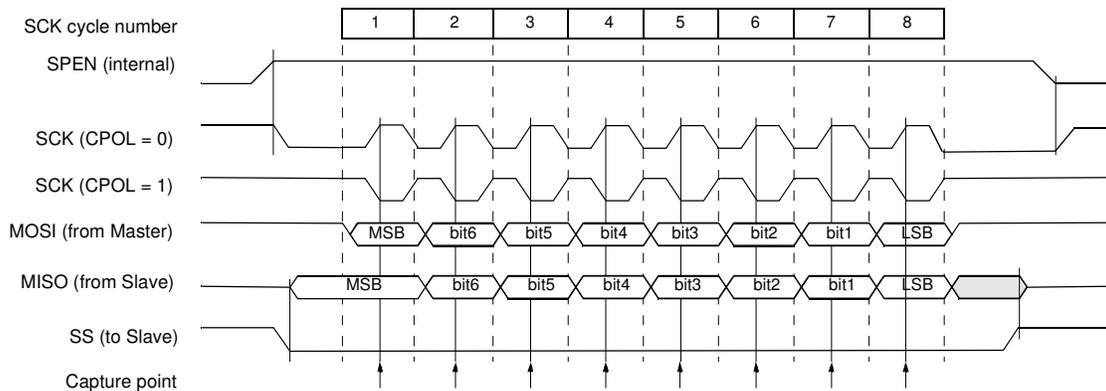
**Figure 46. Data Transmission Format (CPHA = 1)**
