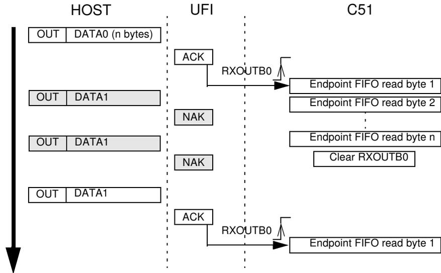
An endpoint will be first enabled and configured before being able to receive Bulk or Interrupt packets.
