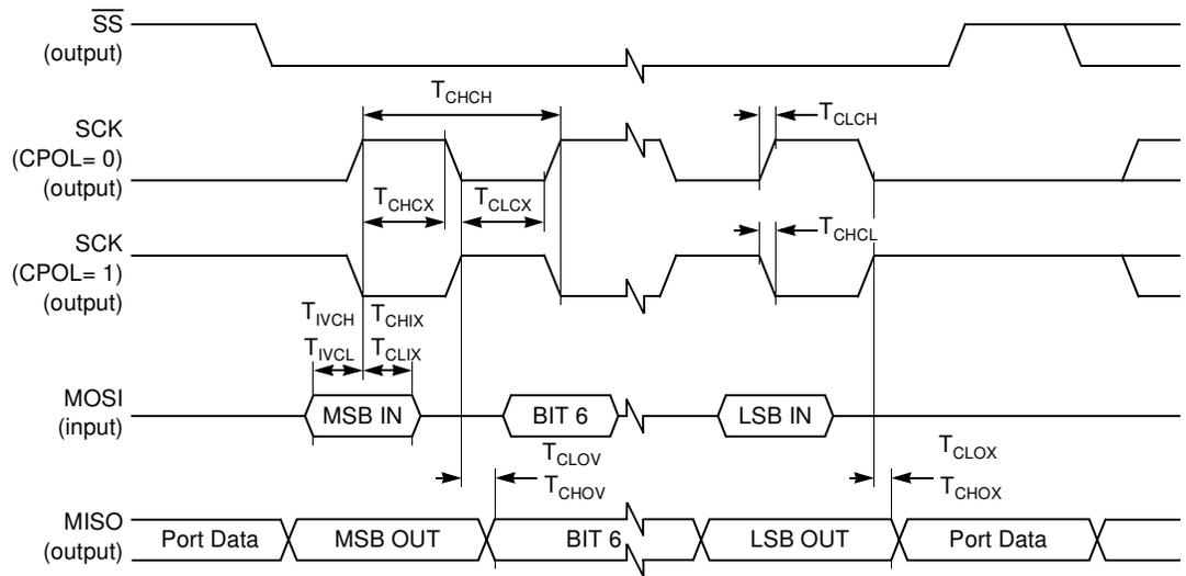
Note: 1.  $\overline{SS}$  handled by software using general purpose port pin.
