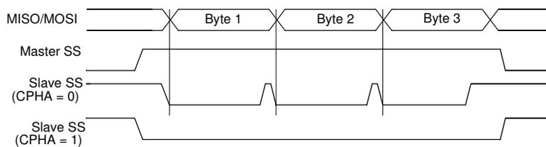
As shown in Figure 46, the first SCK edge is the MSB capture strobe. Therefore the Slave must begin driving its data before the first SCK edge, and a falling edge on the SS pin is used to start the transmission. The SS pin must be toggled high and then low between each byte transmitted (Figure 43).
