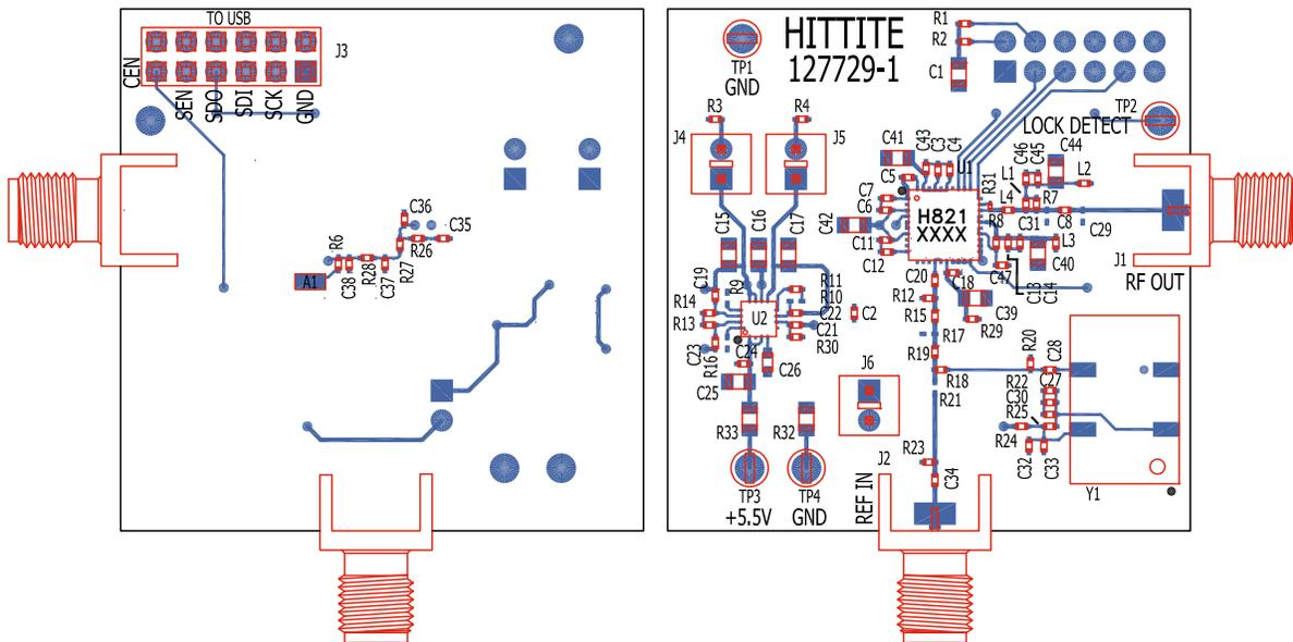
The circuit board used in the application should use RF circuit design techniques. Signal lines should have 50 Ohm impedance while the package ground leads and exposed paddle should be connected directly to the ground plane similar to that shown. A sufficient number of via holes should be used to connect the top and bottom ground planes. The evaluation circuit board shown is available from Hittite upon request.
