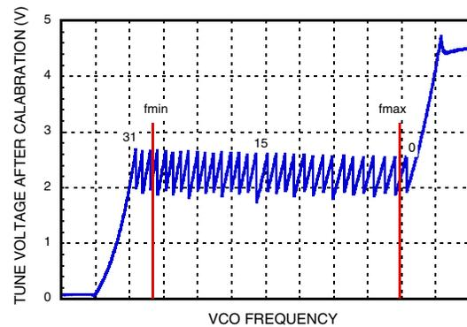
[1] Fractional Mode, 50 MHz Crystal, R=1, ~80 kHz Loop BW, (Loop filter values: Contact factory for component values) 2mA Charge Pump, -385µA Offset.
