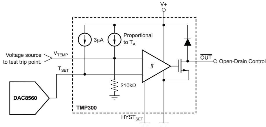
Figure 11. DAC Generates the Voltage-Driving T<sub>SET</sub> Pin
