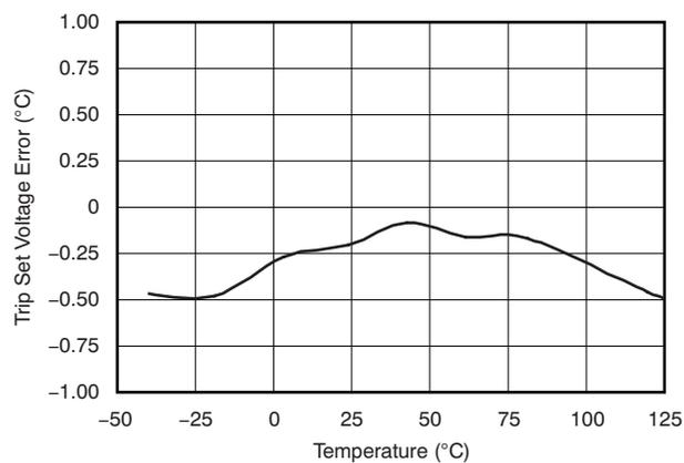
Figure 10. Trip Set Voltage Error vs Temperature
