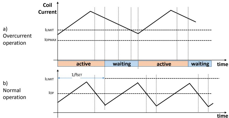
For coil protection purposes, the maximum duty is further limited by the L6364 in relation to the supply voltage so that the maximum coil current rise in one cycle is limited to:
