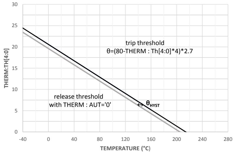
If the trip threshold is exceeded, the output switches are disabled, the event is signaled to the microcontroller via the status register (STATUS:SOT) and an interrupt is generated.
