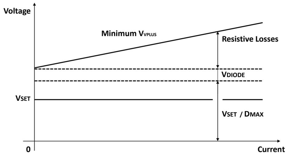
The supply voltage ( $V_{PLUS}$ ) required to reach a nominal output voltage ( $V_{SET}$ ) is given by:
