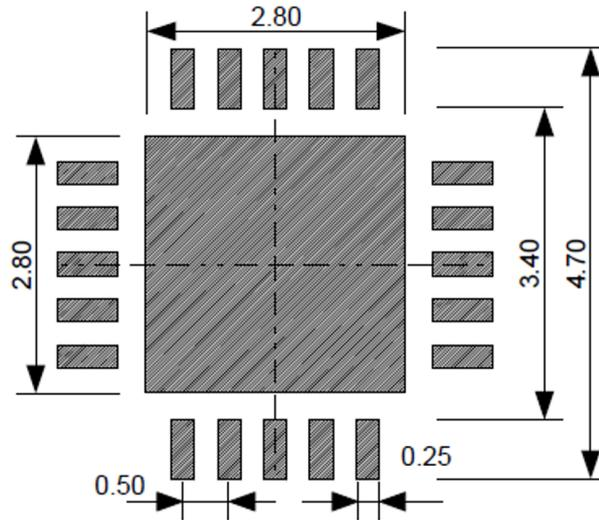
Figure 27. QFN20L, Packing information (drawing and dimension [mm])
