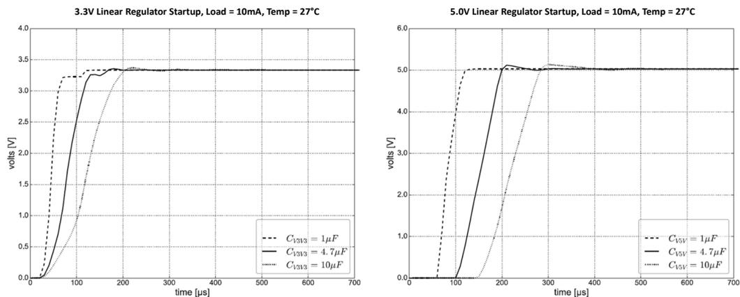
The 5.0 V regulator output is not used internally and is provided for external use. When in use, an external blocking capacitor  $C_{V5V}$  must be provided for stable operation, and the input supply range must be sufficient ( $V_{PLUS} > V_{SUP}$  in pure mode or  $V_{DCDC} > V_{DCDC\_5V\_MIN}$  for DC-DC operation).
