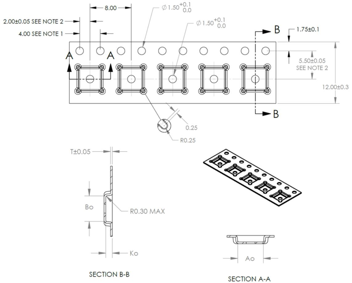
Note: 1: 10 SPROCKET HOLE PITCH CUMULATIVE TOLERANCE  $\pm 0.2$
