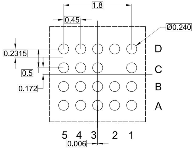
Figure 30. CSP19, Packing Information (drawing and dimension [mm])
