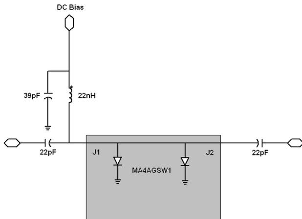
Note: The bias network can be connected to either J1 or J2
