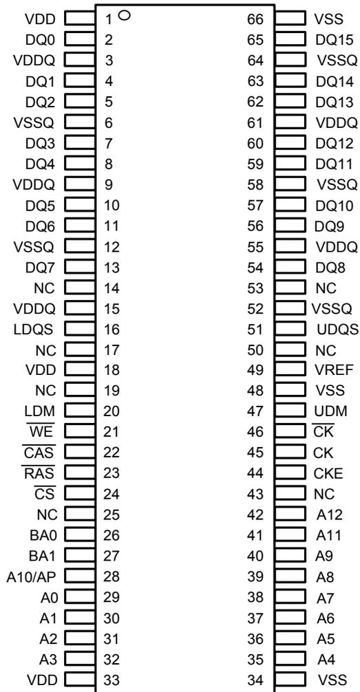
**Figure 1.1 Ball Assignments (Top View)**
