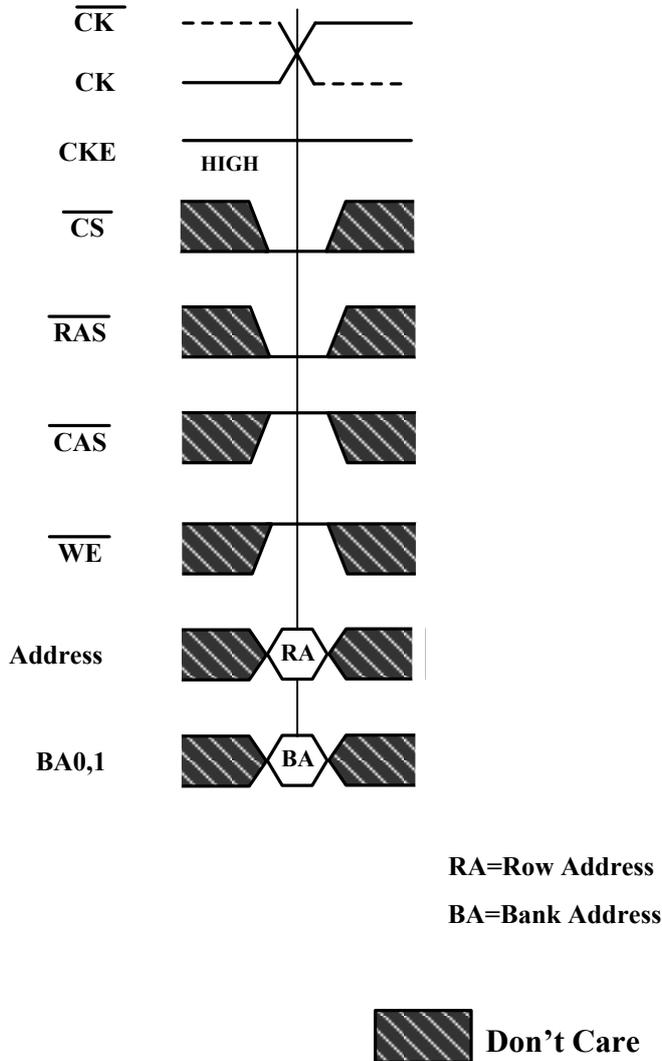
**Figure 5. t<sub>RCD</sub> and t<sub>RRD</sub> Definition**
