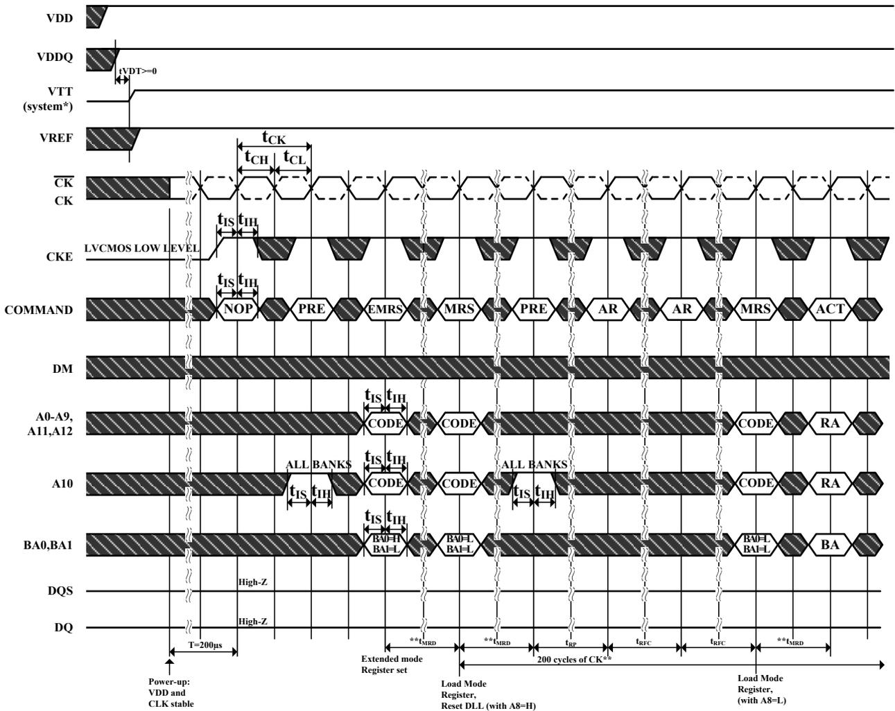
\*=VTT is not applied directly to the device, however  $t_{VTD}$  must be greater than or equal to zero to avoid device latch-up.
