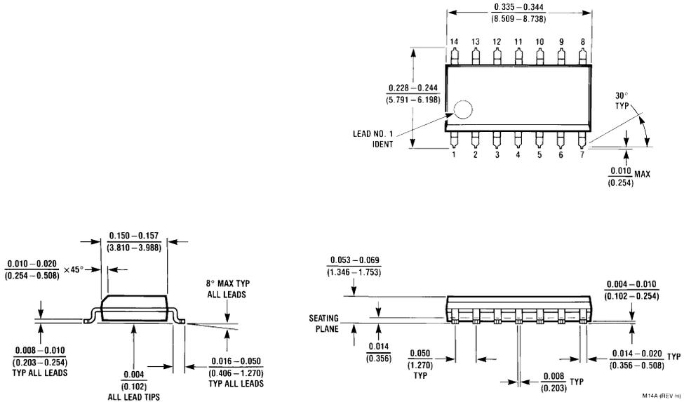
**14-Lead Plastic Dual-In-Line Package (PDIP), JEDEC MS-120, 0.150" Narrow
