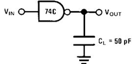
Note: Delays measured with input  $t_r, t_f = 20 \text{ ns}$ .
