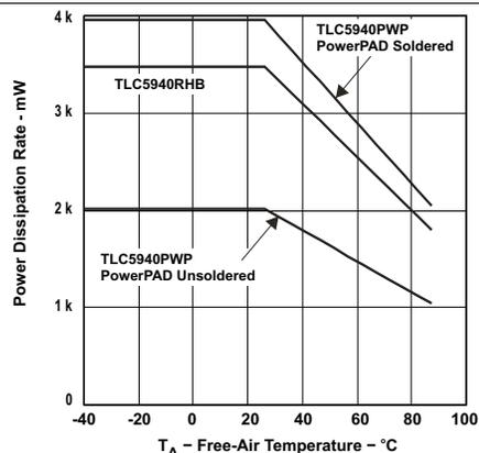
Figure 2. Power Dissipation Rate vs Free-Air Temperature
