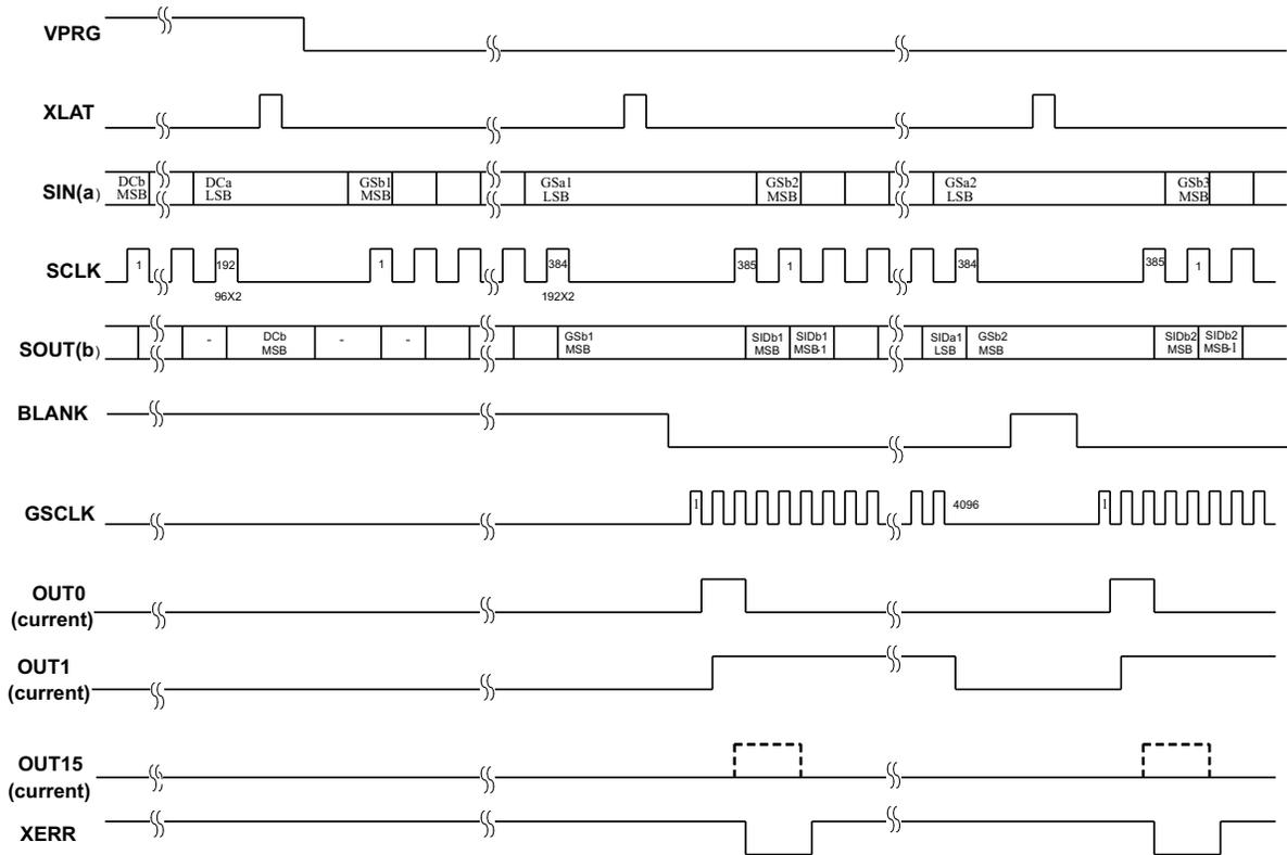
Figure 14. Timing Chart for Two Cascaded TLC5940-EP Devices
