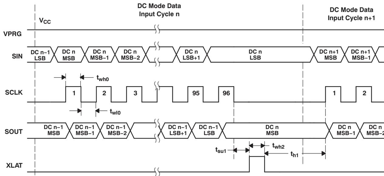
Figure 16. Dot Correction Data Input Timing Chart
