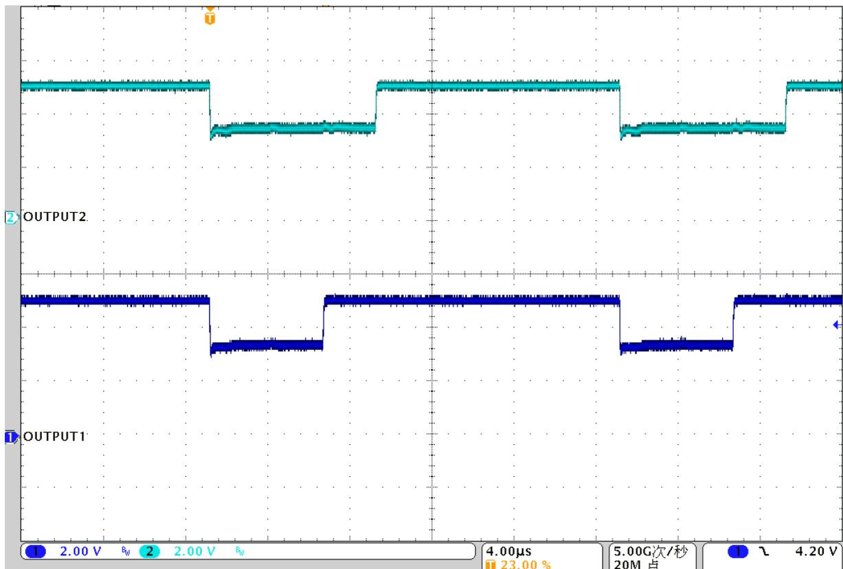
Figure 24. Output Waveform with Different Grayscale PWM Data
