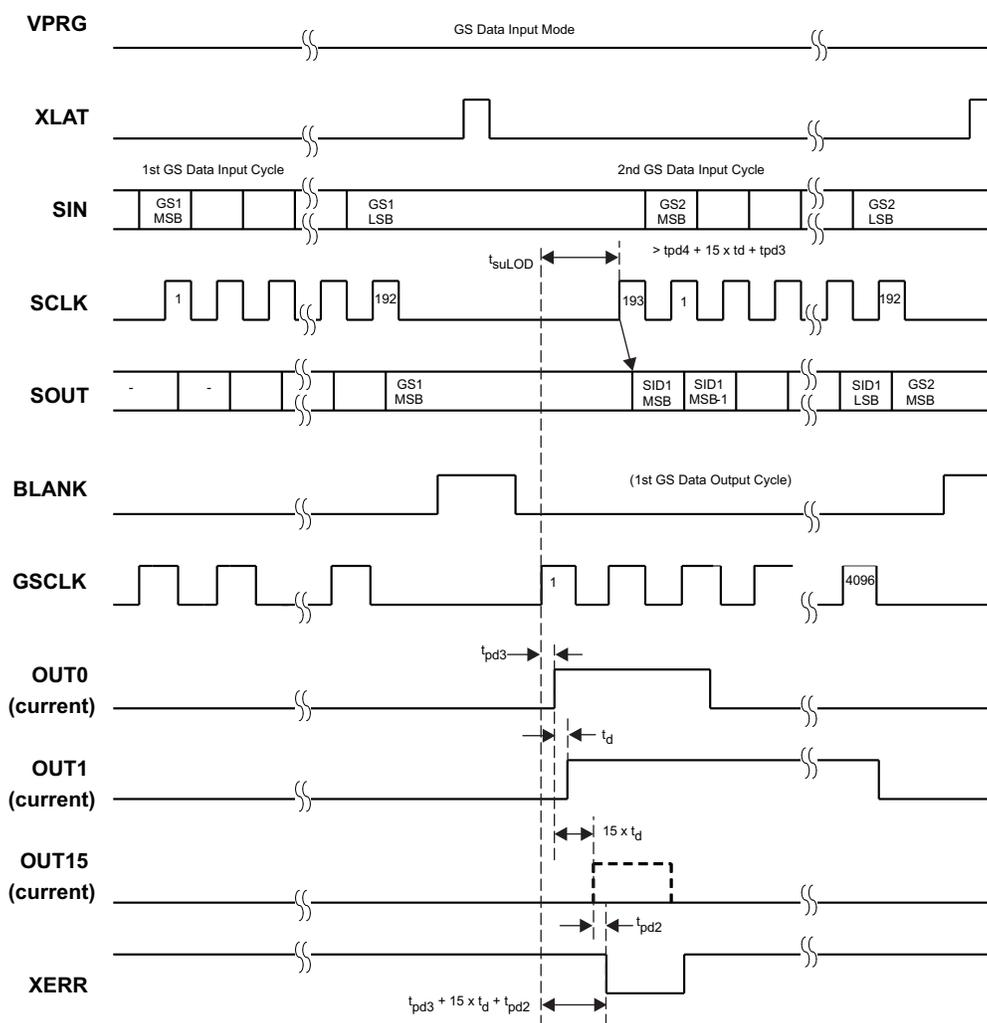
Figure 21. Readout Status Information Data (SID) Timing Chart
