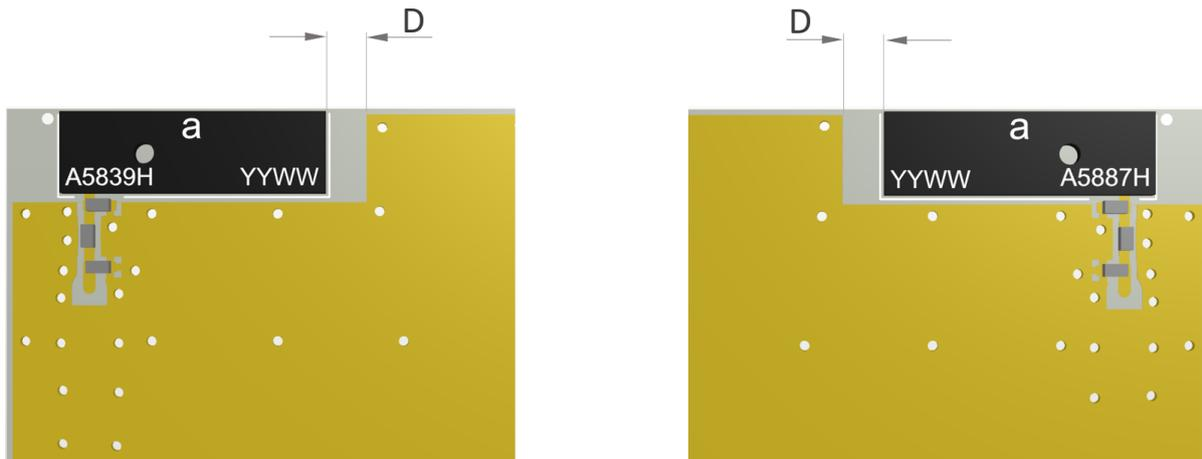
Additional ground and components near the antenna should be at a distance of at least 2mm. Where possible the antenna should be clear of ground from both sides, although the antenna can work well with a minimum clearance of  $D \geq 2$  mm as shown in the drawing above.
