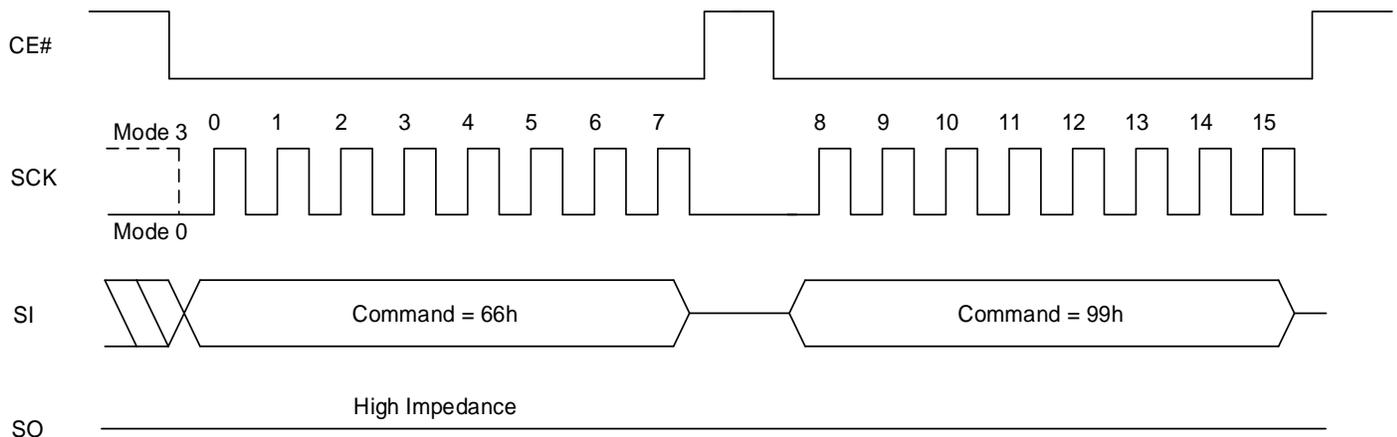
**Figure 8.51 Software Reset Enable and Software Reset Sequence In QPI Mode (RSTEN, 66h + RST, 99h)**
