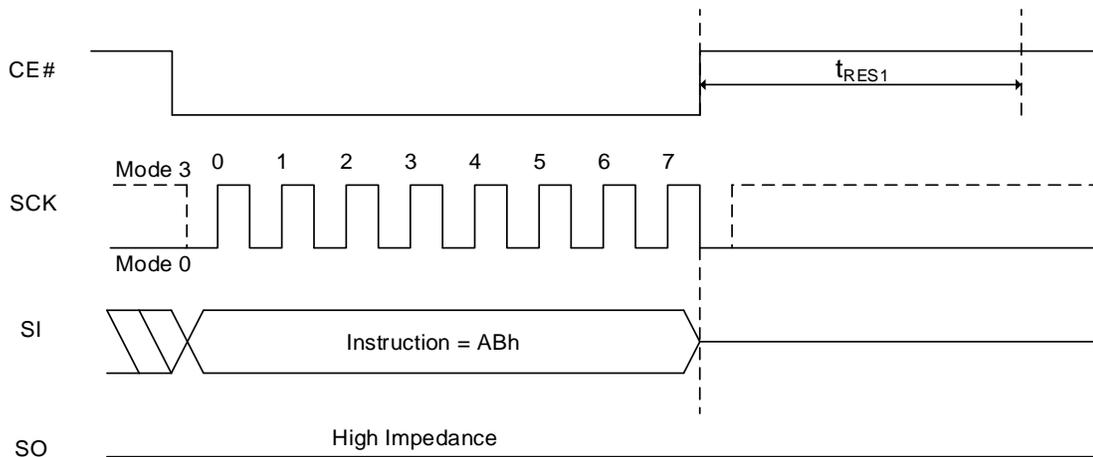
Figure 8.41 Release Deep Power Down Mode Sequence In QPI Mode
