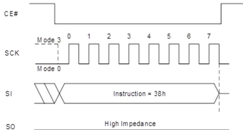
Figure 8.1 Exit Quad Peripheral Interface (QPI) Mode Sequence
