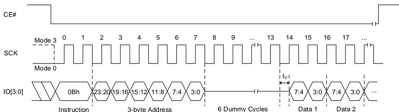
**Note:** Number of dummy cycles can be configured by C0h command
