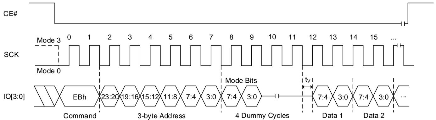
“Wrap Around” feature is not available in QPI mode for Fast Read Quad I/O command. To perform a read operation with fixed data length wrap around in QPI mode, a dedicated “Burst Read with Wrap” (0Ch) command must be used.
