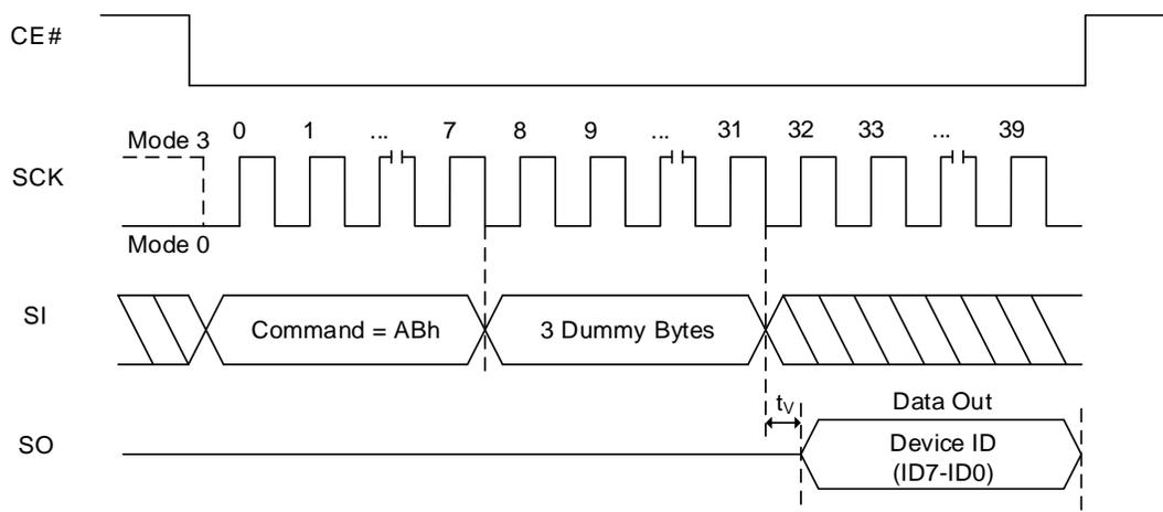
**Figure 8.43 Read Product Identification Sequence In QPI Mode**
