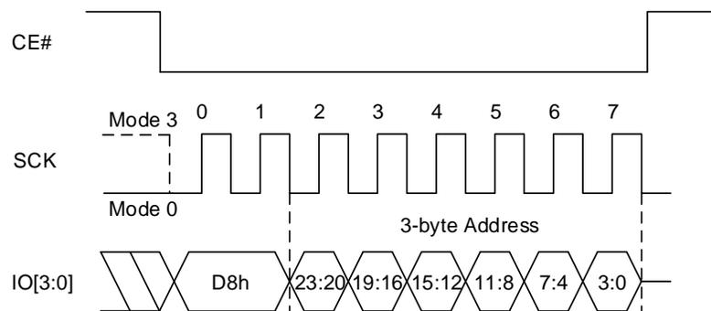
**Figure 8.21 Block Erase (32K) Sequence In SPI Mode**
