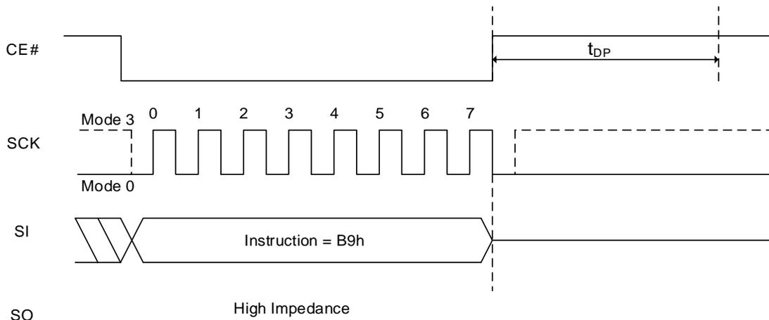
Figure 8.39 Enter Deep Power Down Mode Sequence In QPI Mode
