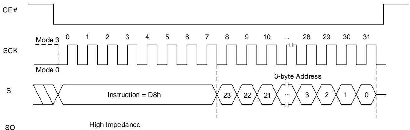
**Figure 8.20 Block Erase (64K) Sequence In QPI Mode**
