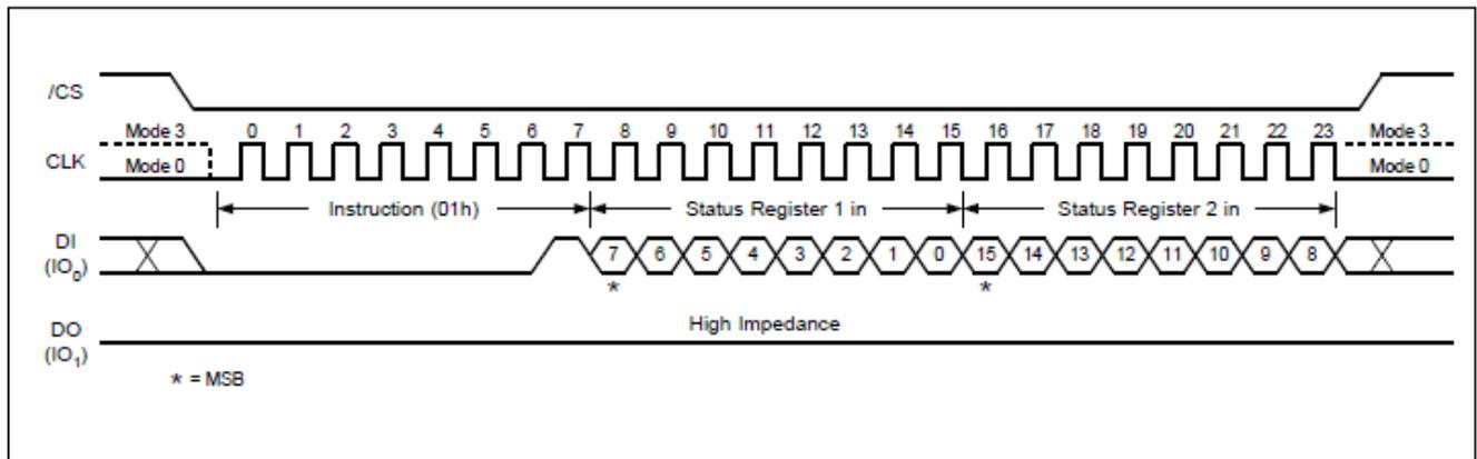
**Figure 8.36 Two Byte Write Status Register Sequence In QPI Mode**
