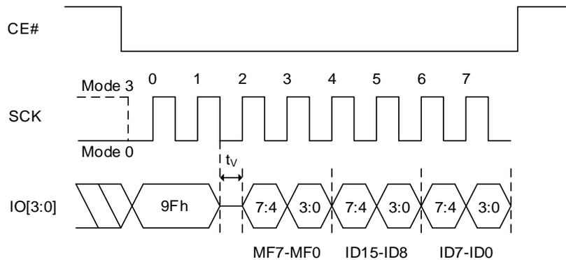
**8.25 READ DEVICE MANUFACTURER AND DEVICE ID OPERATION (RDMDID, 90h)**
