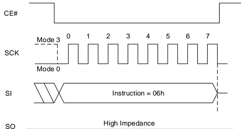
**Figure 8.26 Write Enable Sequence In QPI Mode**
