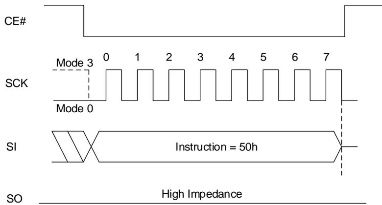
Figure 8.30 Write Enable for Volatile Status Registers Sequence In QPI Mode
