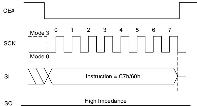
**Figure 8.24 Chip Erase Sequence In QPI Mode**
