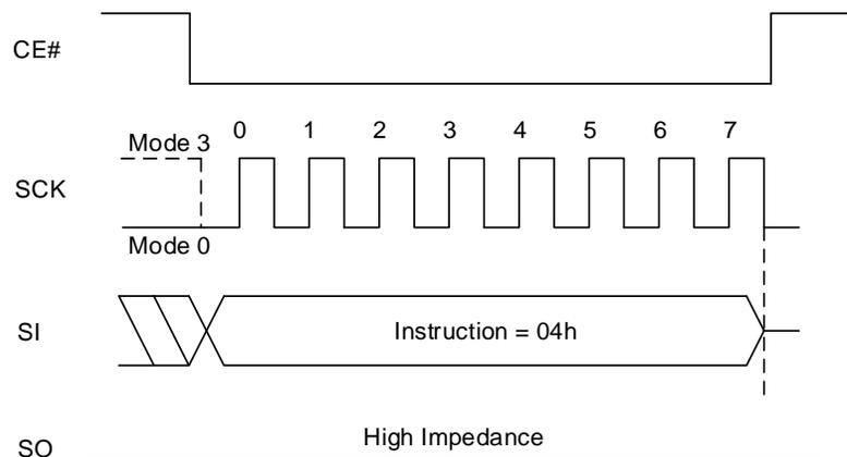
Figure 8.28 Write Disable Sequence In QPI Mode
