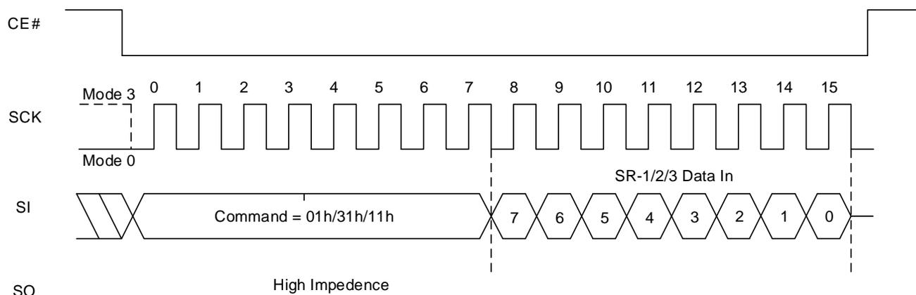
**Figure 8.34 Write Status Register Sequence In QPI Mode**
