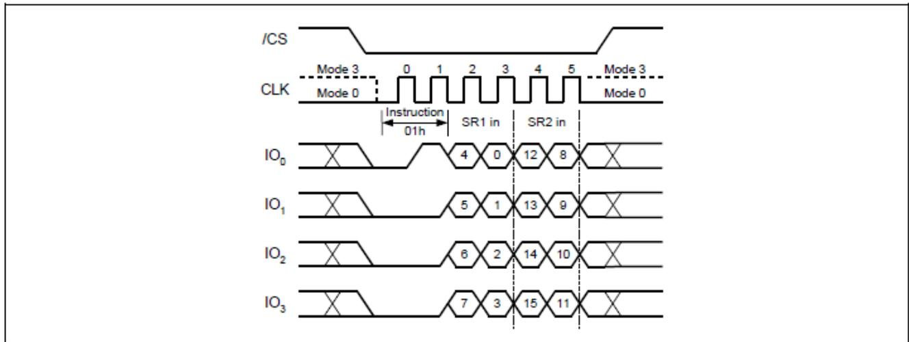
**8.19 ENTER QUAD PERIPHERAL INTERFACE (QPI) MODE OPERATION (QPIEN, 38h; QPIDI, FFh)**
