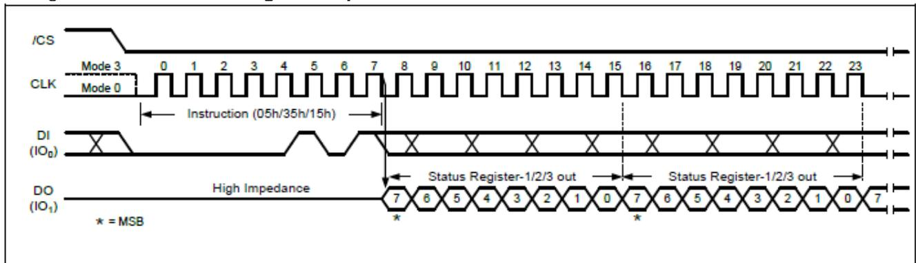
**Figure 8.32 Read Status Register Sequence In QPI Mode**
