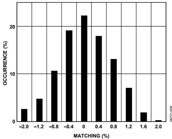
Figure 8. Excitation Current Matching (210 µA) at Ambient Temperature
