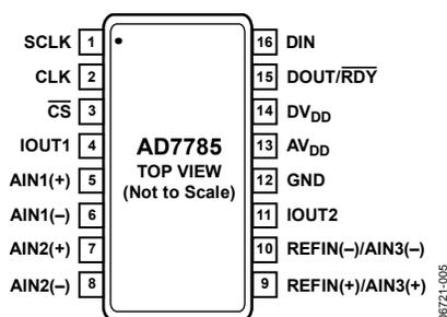
Figure 5. Pin Configuration
