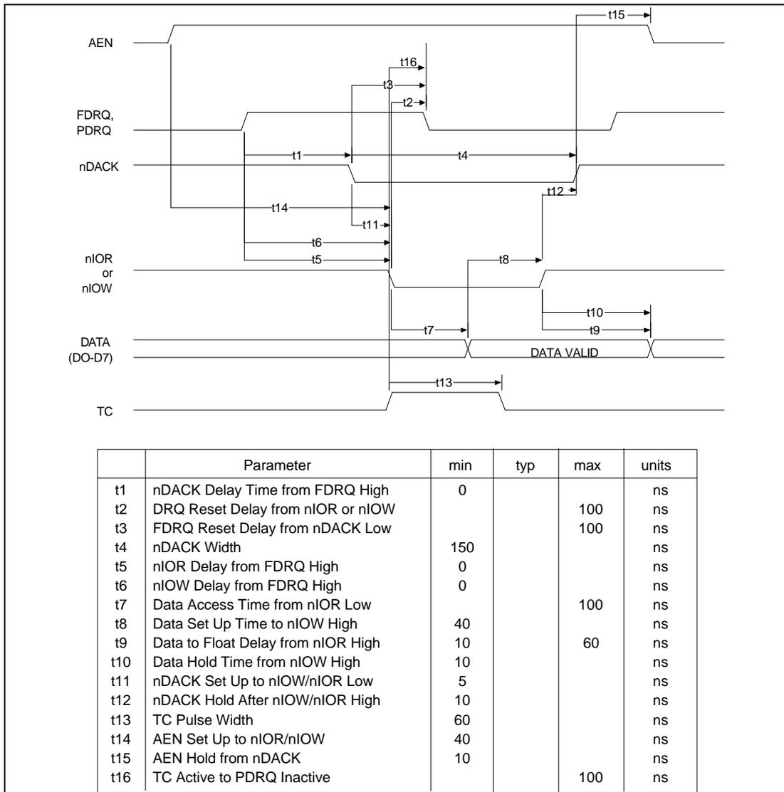
**FIGURE 6 - DMA TIMING**
