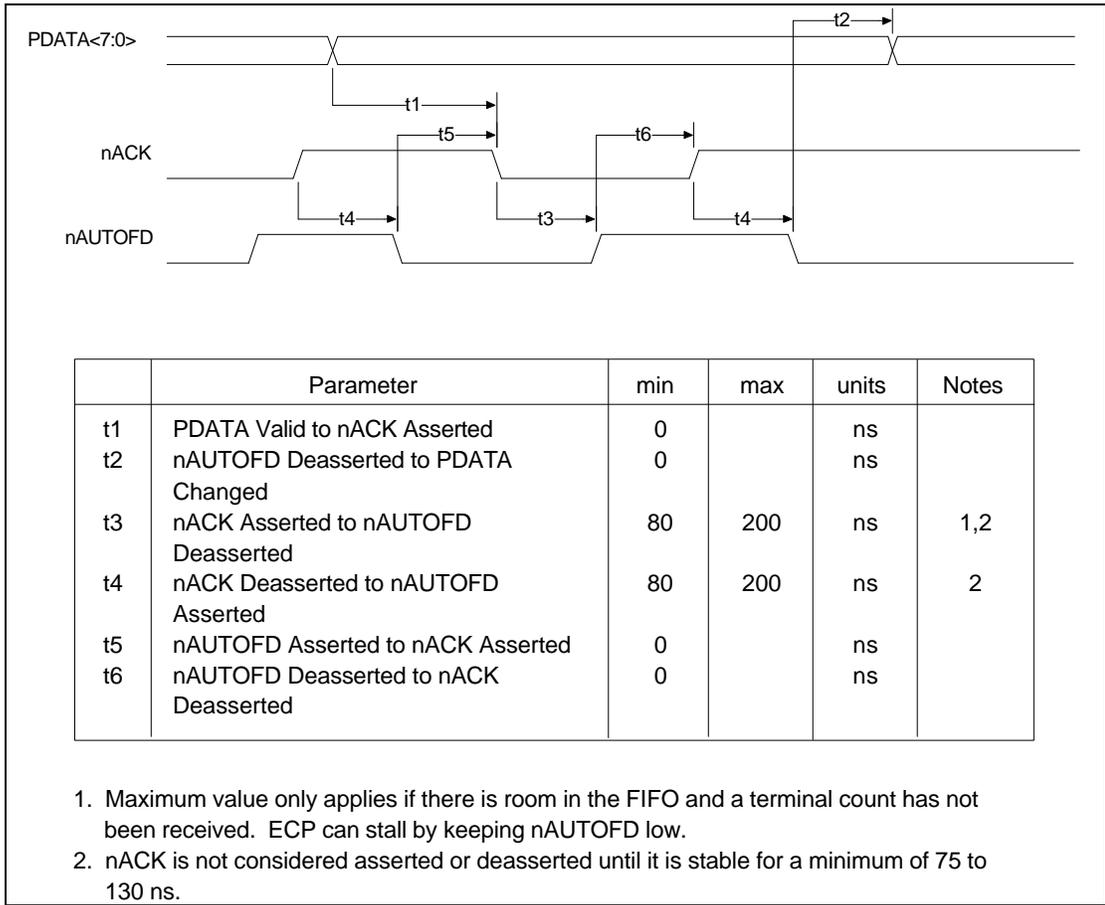
**FIGURE 19 - ECP PARALLEL PORT REVERSE TIMING**
