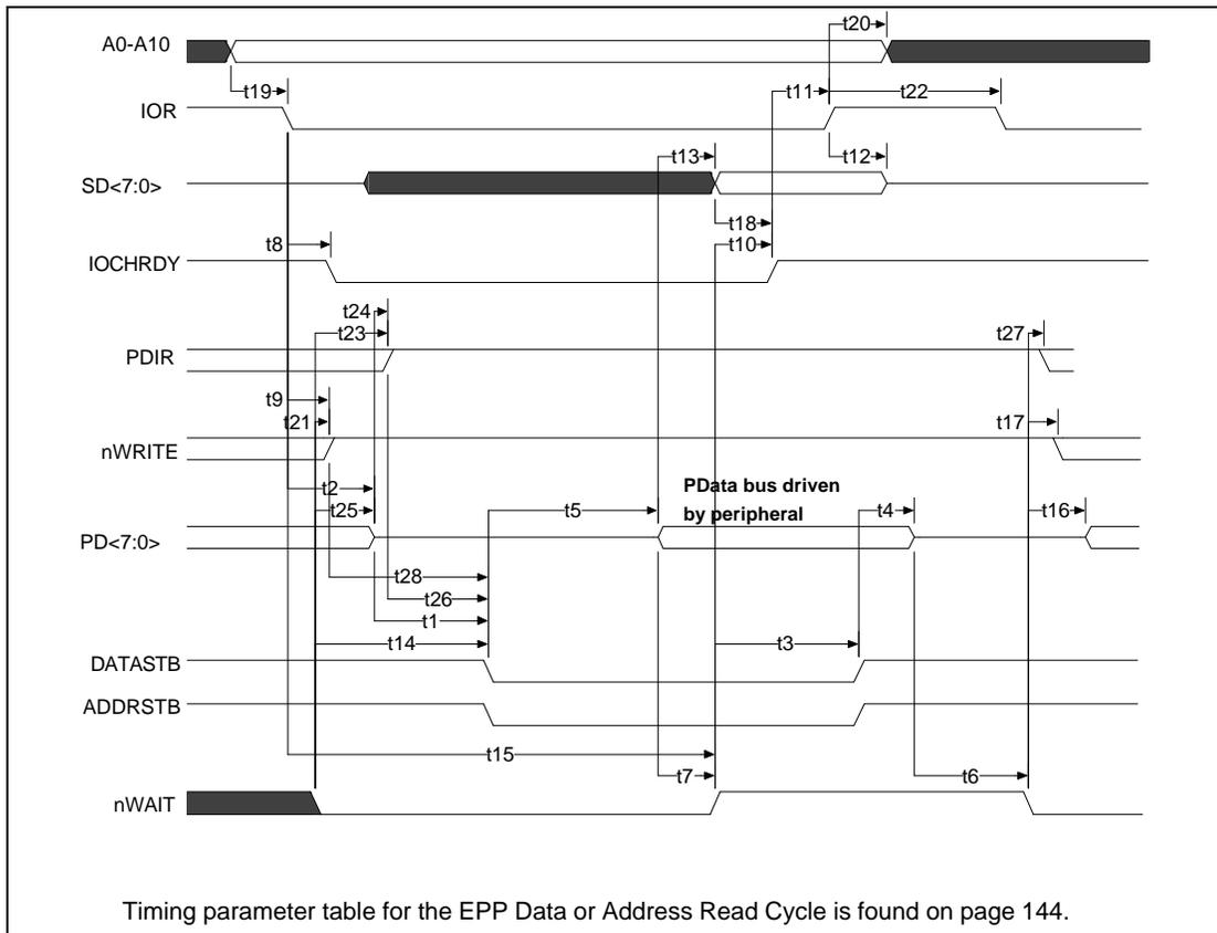
**FIGURE 14A - EPP 1.9 DATA OR ADDRESS READ CYCLE**
