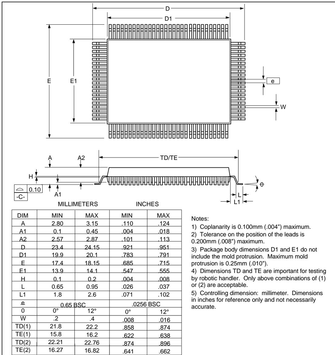
FIGURE 20 - 100 PIN QFP
