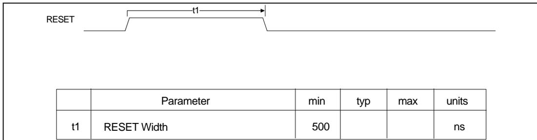
**FIGURE 7 - RESET TIMING**
