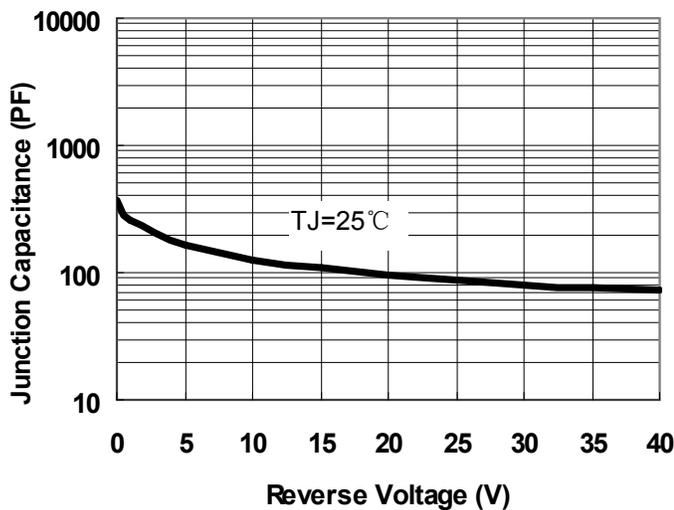
Fig.1-Typical Junction Capacitance
