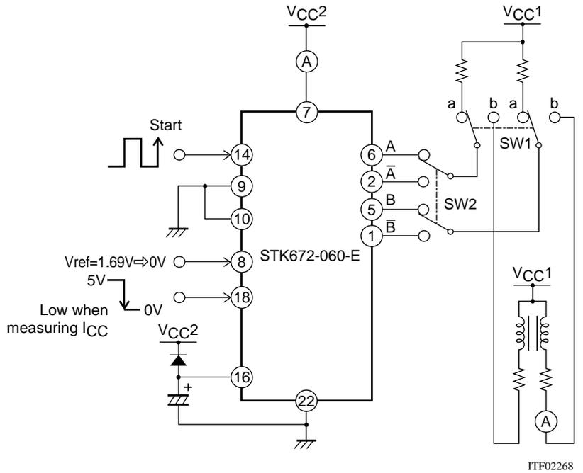
When measuring I<sub>oave</sub>: With SW1 set to 'b', V<sub>ref</sub> = 1.69V
