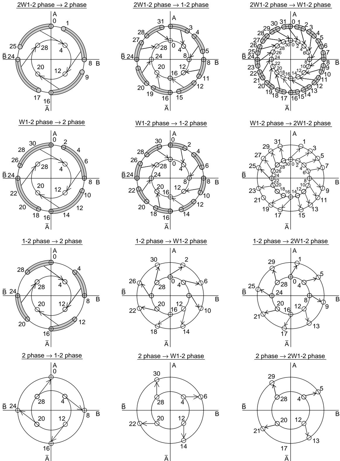
Excitation phase developed by the first CLK internal pulse after the change in the excitation mode setting with M1 and M
