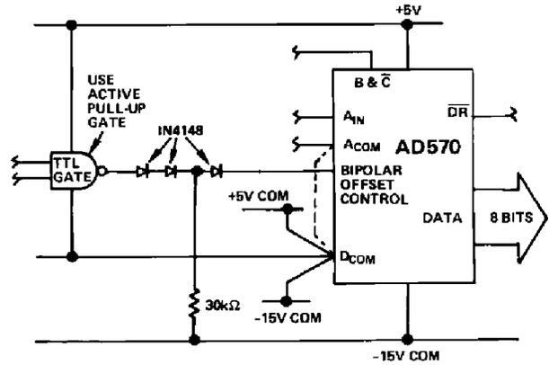
Figure 5. Bipolar Offset Controlled by Logic Gate
