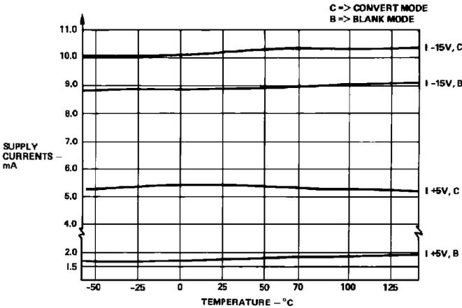
Figure 2. AD570 Power Supply Current vs. Temperature
