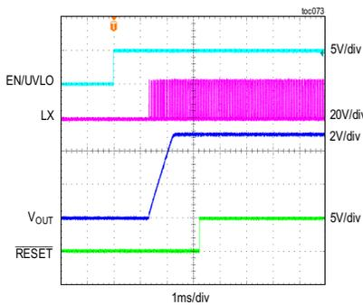
MAXM17634/MAXM17635 SHUTDOWN THROUGH ENABLE
