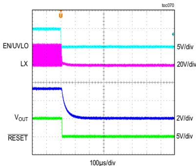
MAXM17633/MAXM17635 STARTUP THROUGH ENABLE
