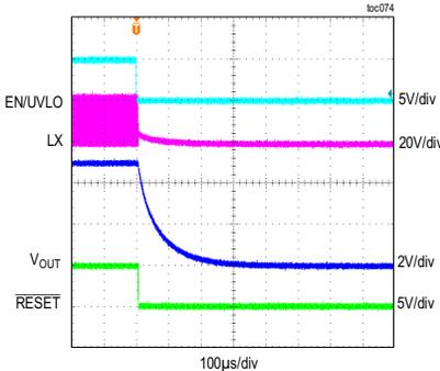
MAXM17634/MAXM17635 STARTUP THROUGH ENABLE
