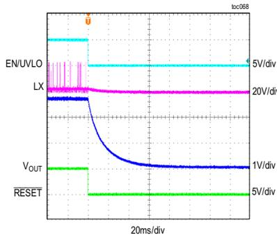
MAXM17633/MAXM17635 STARTUP THROUGH ENABLE
