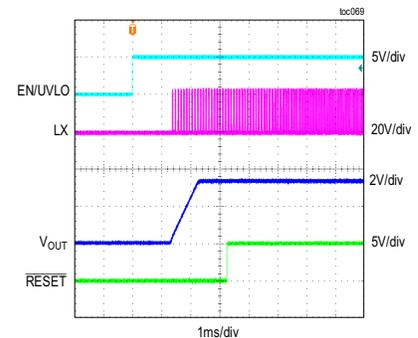
MAXM17633/MAXM17635 SHUTDOWN THROUGH ENABLE
