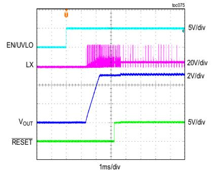
MAXM17634/MAXM17635 SHUTDOWN THROUGH ENABLE
