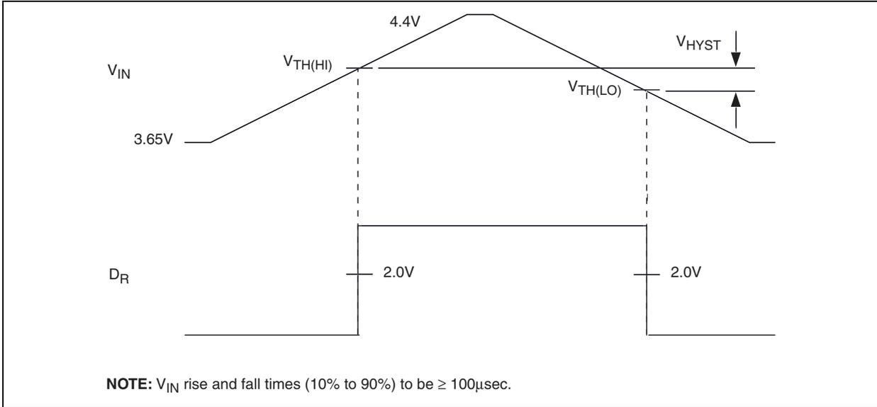
**FIGURE 4-2: TIMING DIAGRAM**
