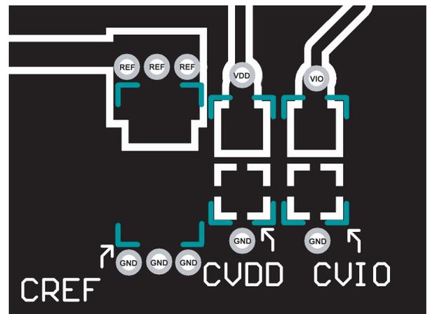
Figure 43. Example Layout of the [AD7980](#) (Bottom Layer)
