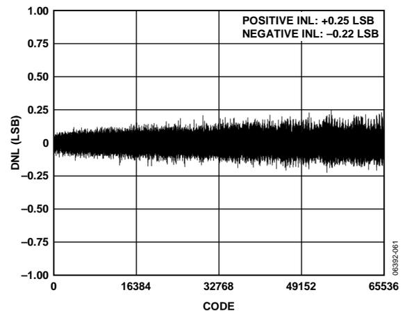
Figure 9. Differential Nonlinearity vs. Code, REF = 2.5 V
