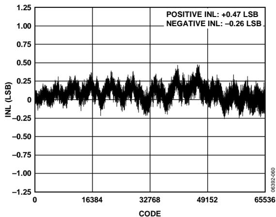
Figure 6. Integral Nonlinearity vs. Code, REF = 2.5 V
