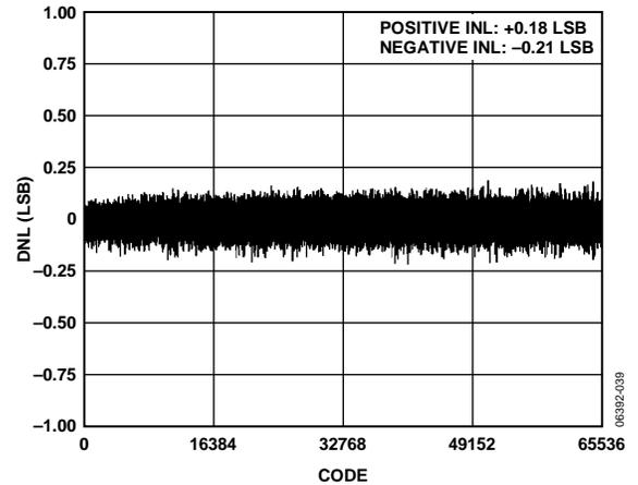
Figure 8. Differential Nonlinearity vs. Code, REF = 5 V
