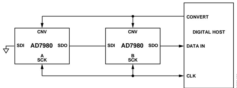
Figure 38. Chain Mode Without Busy Indicator Connection Diagram
