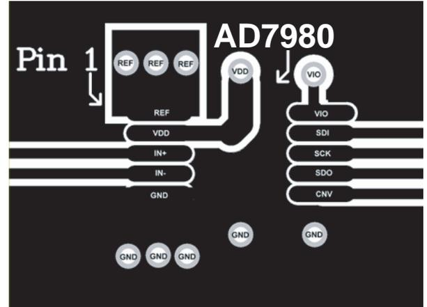
Figure 42. Example Layout of the [AD7980](#) (Top Layer)
