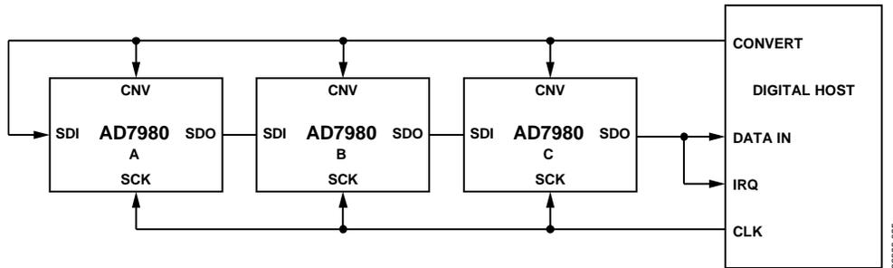
Figure 40. Chain Mode with Busy Indicator Connection Diagram
