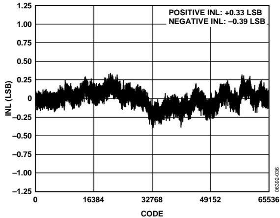
Figure 5. Integral Nonlinearity vs. Code, REF = 5 V
