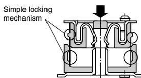
Simple locking mechanism
