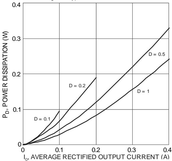
Figure 3 Forward Power Dissipation,  $T_J = 125^\circ\text{C}$
