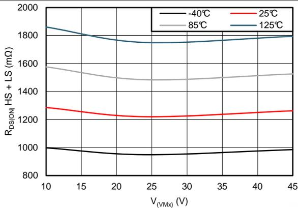
Figure 3.  $R_{DS(ON)}$  vs  $V_{VMx}$
